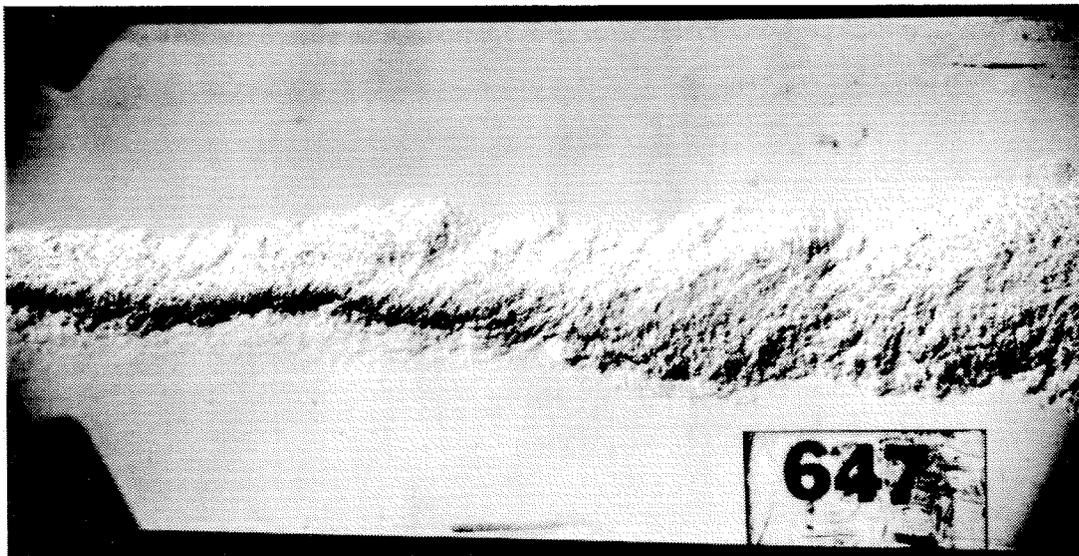
Figure C.33: Schlieren photograph of Case 3h flow (Run 647). Upper stream is high-speed, reactant-rich ( $\phi = 1/8$ ).
