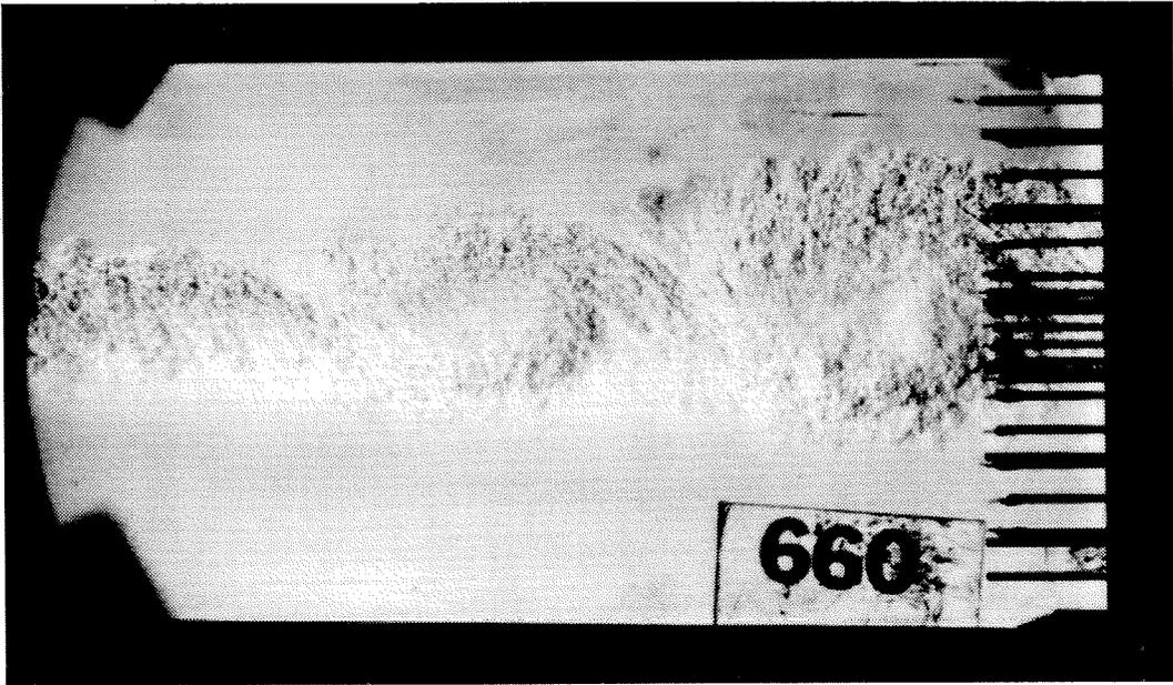
Figure C.49: Schlieren photograph of Case 4f flow (Run 660). Upper stream is low-speed, reactant-lean ( $\phi = 1/8$ ).
