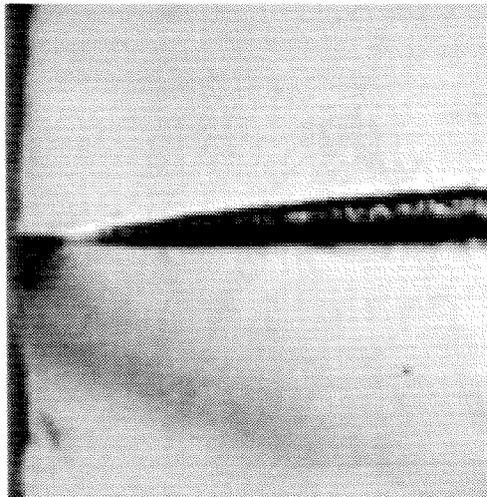
Figure C.48: Magnified (3x) schlieren photograph of splitter-plate region of Case 4f flow (Run 661). Upper stream is low-speed, reactant-lean ( $\phi = 1/8$ ). Notice that the shear layer is growing into the upper stream.
