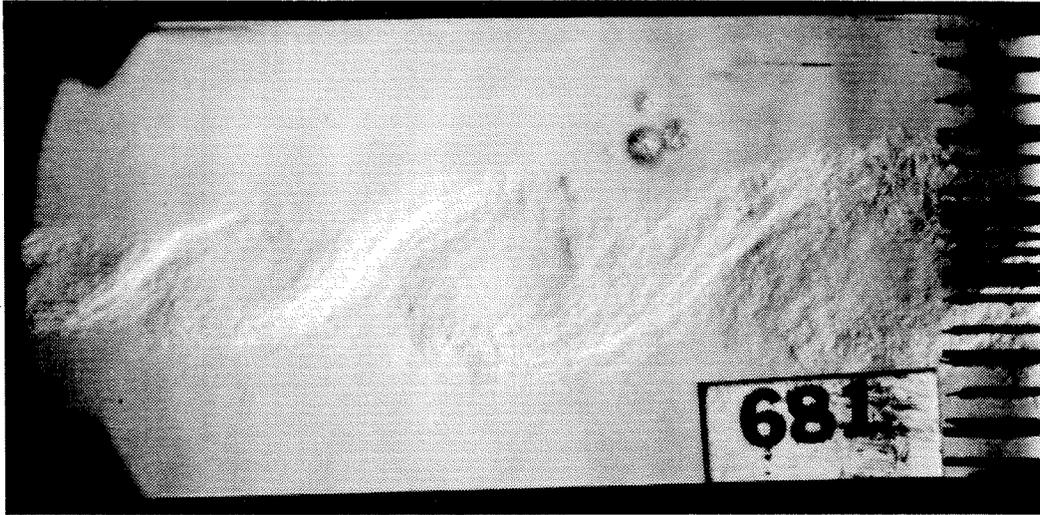
Figure C.2: Schlieren photograph of Case 1c flow. For contrast, a mixture of C<sub>2</sub>H<sub>4</sub>, He and Ar was used on the upper stream to replace N<sub>2</sub>.
