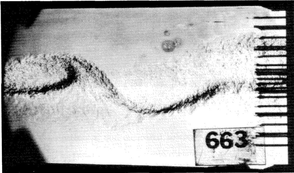
Figure 4.8: Schlieren image of case 4h flow. Flagellation of the layer is clearly visible. The lower stream is the high-speed stream.
