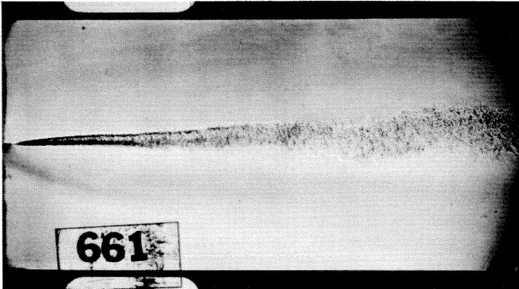
Figure C.47: Schlieren photograph of upstream portion of Case 4f flow (Run 661). Upper stream is low-speed, reactant-lean ( $\phi = 1/8$ ).
