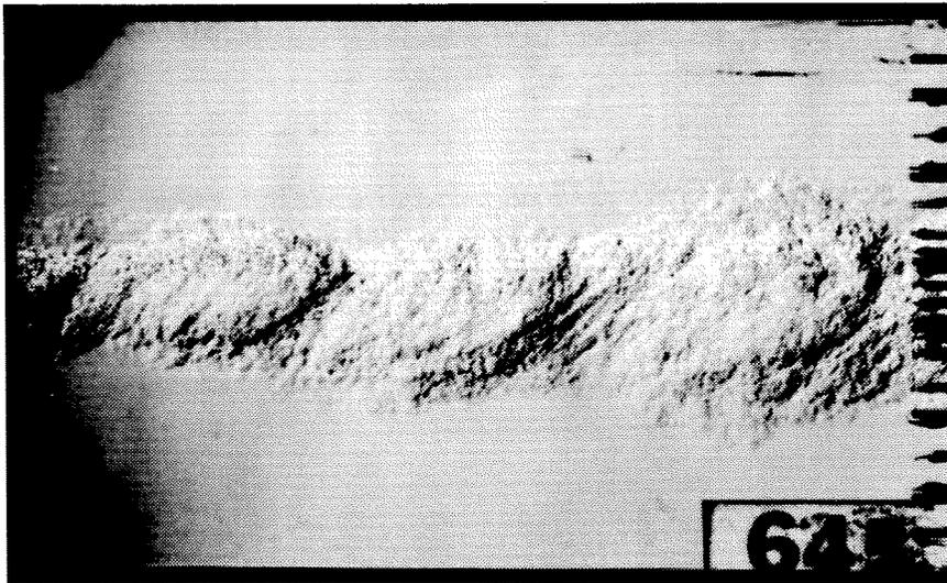
Figure C.37: Schlieren photograph of Case 3f flow (Run 645). Upper stream is high-speed, reactant lean ( $\phi = 1/8$ ).
