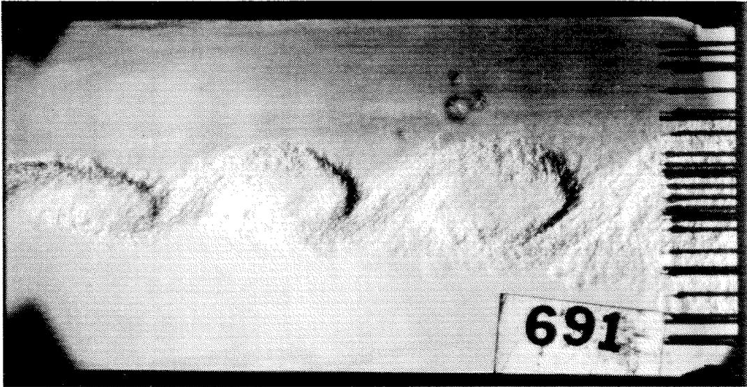
Figure C.10: Schlieren photograph of Case 1f flow (Run 691). Upper stream is high-speed, reactant lean ( $\phi = 8$ ).
