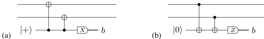
Figure 3.3: Ideal circuits used to measure weight-two stabilizers: (a) X -type and (b) Z -type. The bottom line represents an ancilla qubit, which is prepared in either |0\rangle or |+\rangle state. In our simulations we assume that every component of the circuits is affected by noise.
