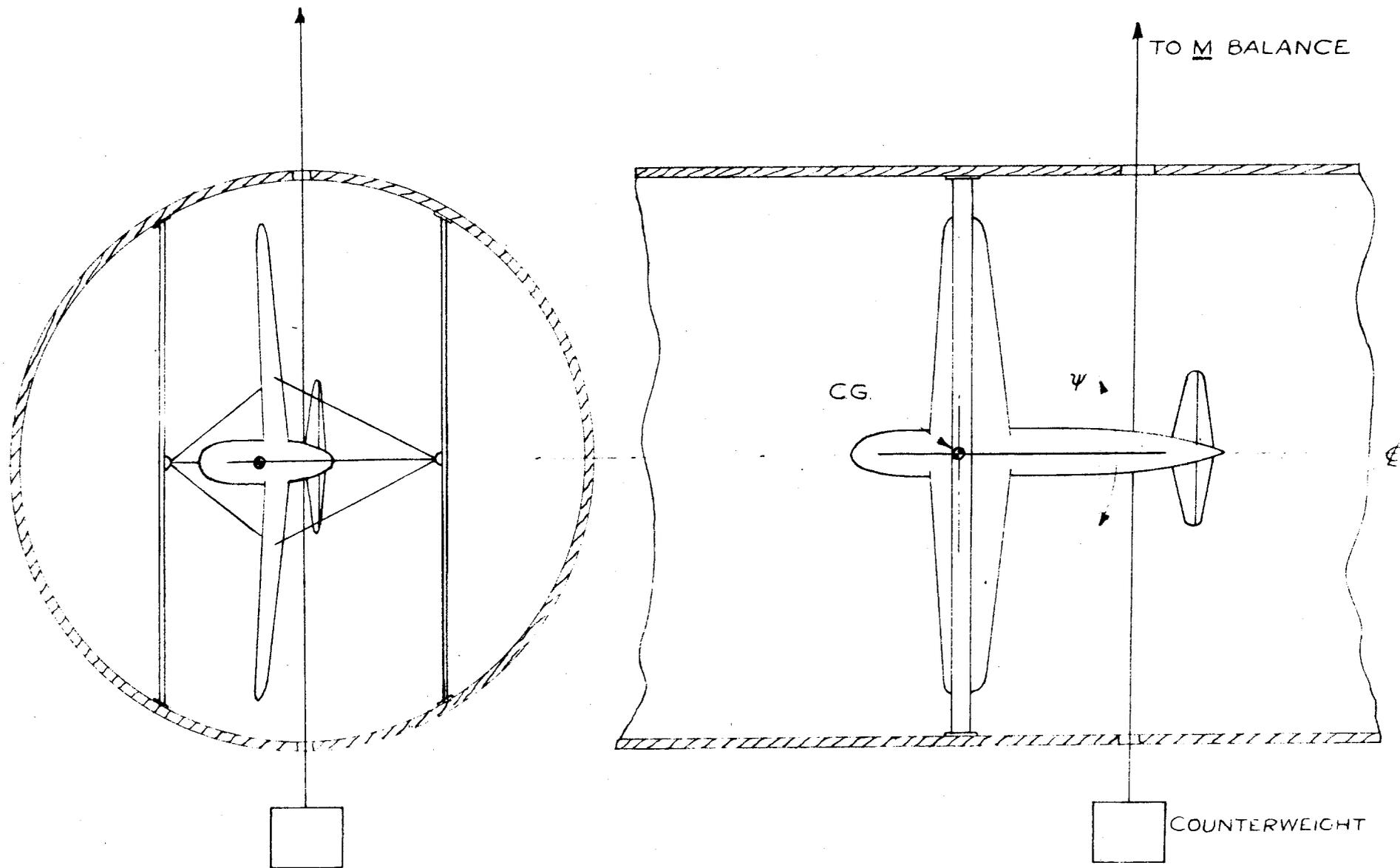
DIAGRAM SHOWING RIGGING FOR YAW-AT-YAW
