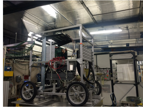
(b) The cart that was used to align the detectors with the beamline.
