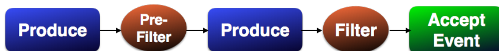
Figure 4.1: Typical HLT path structure. Producers perform physics object reconstruction using the raw event data as input. Filters reject the event if it does not meet specified requirements. A real HLT path may proceed through many stages of production and filtering operations before its final trigger decision is made (only two such stages are depicted here).
