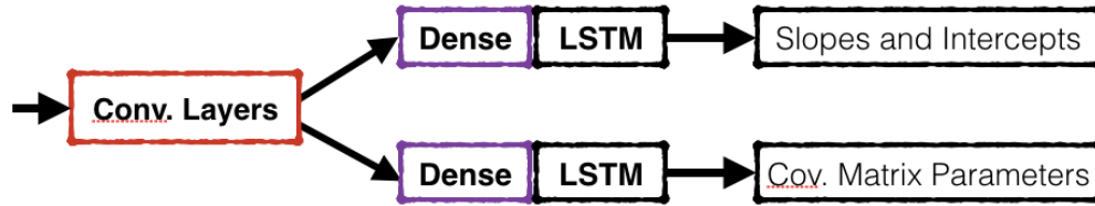
Figure B.12: Diagram of the NN architecture used to identify track parameters and uncertainties in multi-track events.
