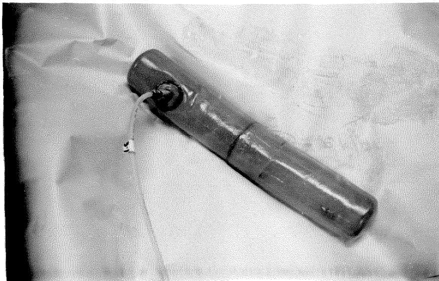
Figure 7.10 Side Pressure-Cell with Attached Aluminum Valve Core, Three-Dimensional Compression Apparatus
