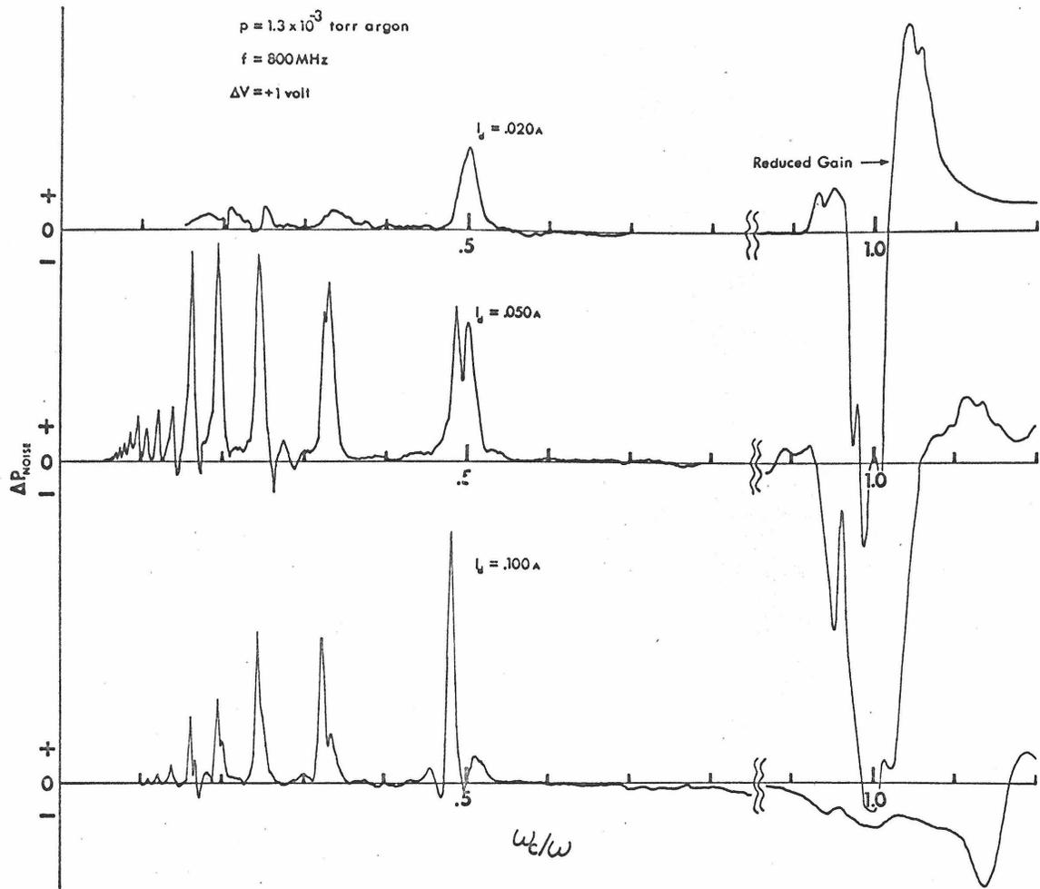
Figure 6.4 Experimental effect of varying the center wire bias
