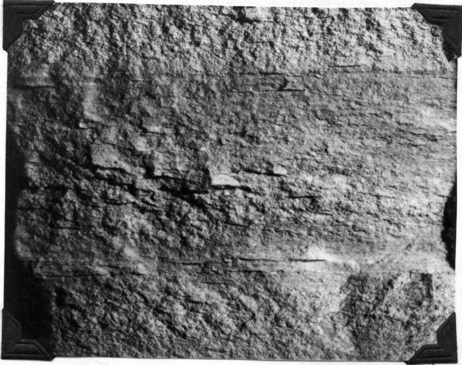
X 5 Slightly Silicified Tuff (somewhat more indurated than Fig. 22. S15, T5S, R14W
