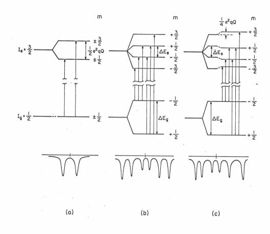
Fig. 4. Nuclear energy levels of Fe<sup>57</sup> and resulting Mössbauer spectra: (a) Electric quadrupole interaction. (b) Magnetic hyperfine interaction.
