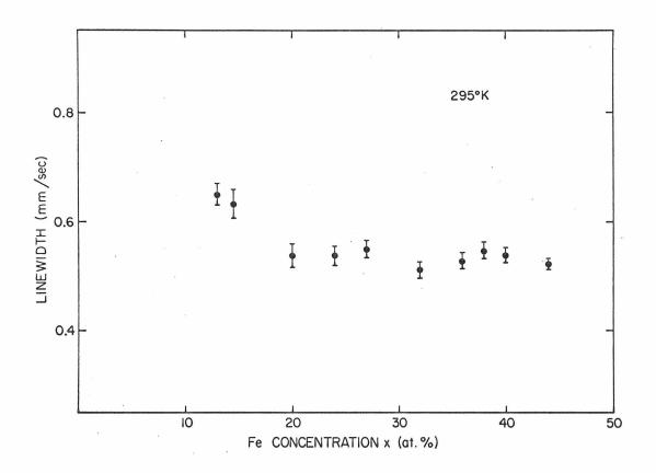
Fig. 8. Linewidth vs. iron concentration for the amorphous  $Fe_x Pd_{80-x}P_{20}$  alloys.
