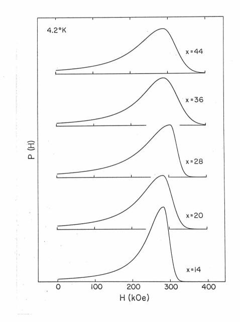
Fig. 12. Hyperfine field distributions corresponding to the fittings of Fig. 11. The vertical scale is the same for all the curves.
