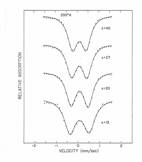
Fig. 5. Typical Mössbauer spectra for the amorphous  $Fe_{x}Pd_{80-x}P_{20}$  alloys at room temperature (295°K).
