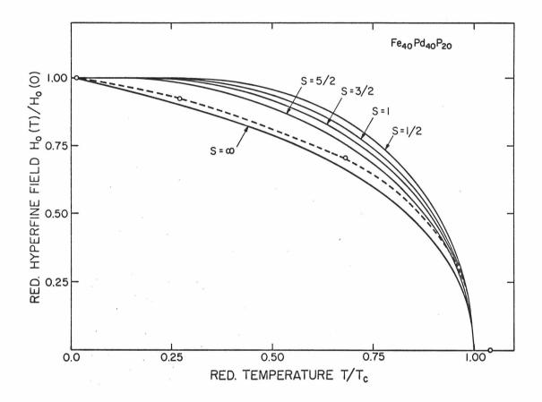
Fig. 34. Reduced (average) hyperfine field vs. temperature for the  $\text{Fe}_{40}\text{Pd}_{40}\text{P}_{20}$  alloy (dashed line).
