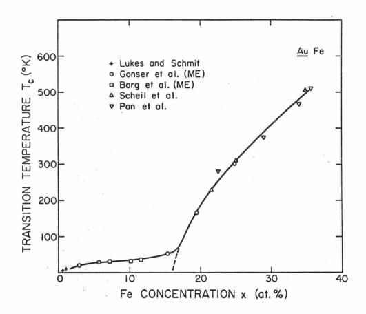
Fig. 41. Magnetic transition temperature vs. iron concentration in Au<sub>1-x</sub> Fe<sub>x</sub> alloys.
