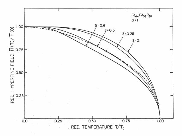
Fig. 37. Comparison of experimental results (dashed line) with Eq. (54) for the Fe<sub>44</sub>Pd<sub>36</sub>P<sub>20</sub> alloy.
