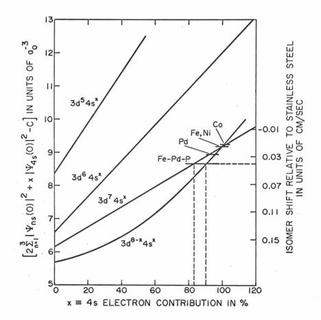
Fig. 30. Isomer shift of Fe<sup>57</sup> in various configurations. (Ref. 41)
