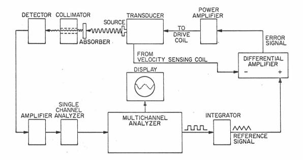
Fig. 1. Schematic diagram of Mössbauer effect apparatus.
