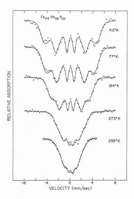
Fig. 18. Temperature dependence of the Mössbauer spectrum for the amorphous  $\text{Fe}_{44}\text{Pd}_{36}\text{P}_{20}$  alloy. The solid curves are the fittings based on Eq. (32).
