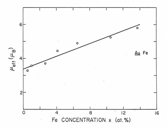
Fig. 40. Effective magnetic moment per Fe atom from susceptibility measurements in Au<sub>1-x</sub> Fe alloys. (Ref. 66)
