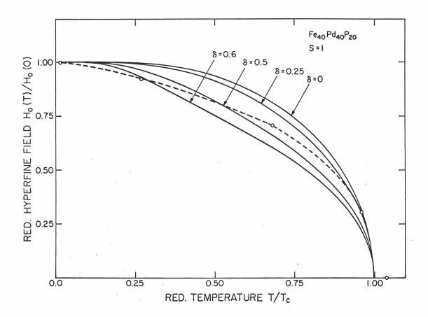
Fig. 38. Comparison of experimental results (dashed line) with Eq. (54) for the  $\text{Fe}_{40}\text{Pd}_{40}\text{P}_{20}$  alloy.
