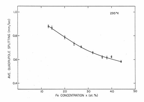
Fig. 7. Quadrupole splitting vs. iron concentration for the amorphous  $Fe_x Pd_{80-x}P_{20}$  alloys.
