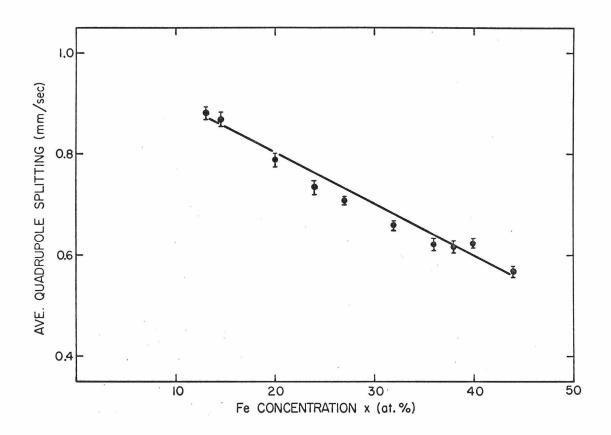
Fig. 36. Quadrupole splitting vs. iron concentration according to Eq. (50).
