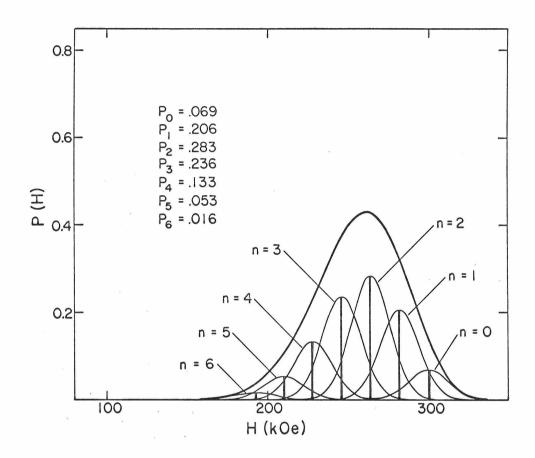
Fig. 10. Illustration of possible hyperfine field distribution in an amorphous material.
