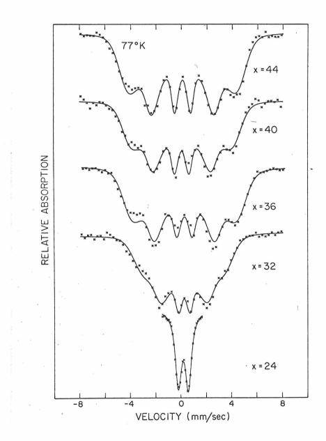
Fig. 13. Mössbauer spectra of the amorphous  $\text{Fe}_{x}^{Pd} \frac{\text{Pd}_{80-x}^{P}}{20}$  alloys at 77°K.
