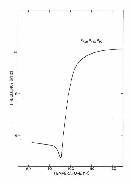
Fig. 26. Frequency measurement for the Fe<sub>28</sub>Pd<sub>52</sub>P<sub>20</sub> alloy.
