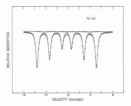
Fig. 2. Example of velocity calibration spectrum taken with a .001" Fe foil.
