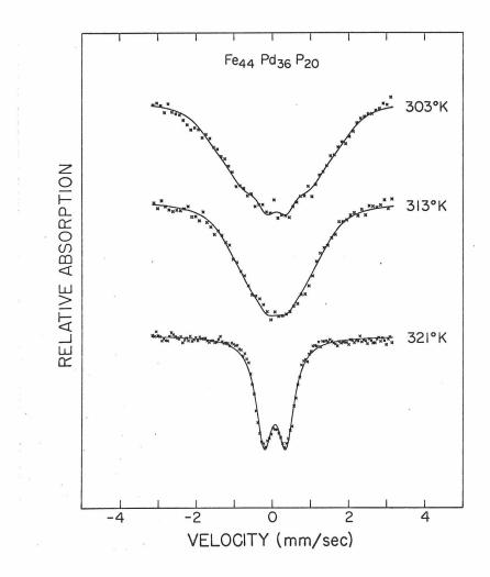
Fig. 20. Mössbauer spectra of the  $\text{Fe}_{44}\text{Pd}_{36}\text{P}_{20}$  alloy near the transition temperature.
