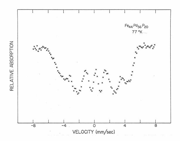
Fig. 9. Low temperature Mössbauer spectrum for the  $Fe_{44}Pd_{36}P_{20}$  alloy.
