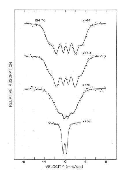
Fig. 15. Mössbauer spectra of the amorphous  $\operatorname{Fe}_{x} \operatorname{Pd}_{80-x} \operatorname{P20}_{20}$  alloys at 194°K.
