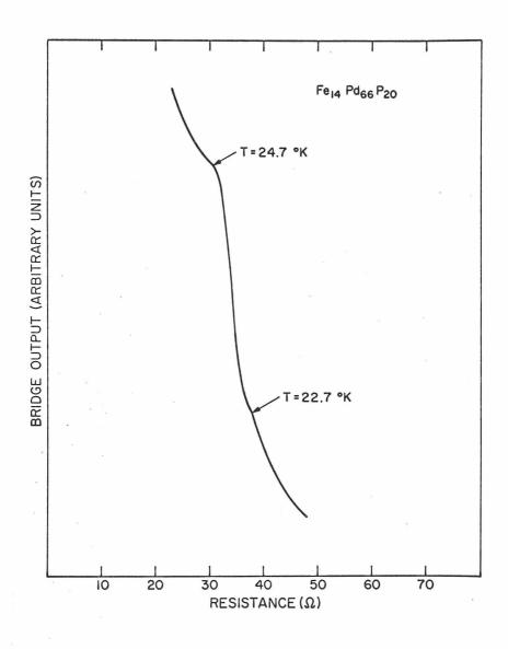
Fig. 28. Output of inductance bridge vs. temperature for the  $\text{Fe}_{14}\text{Pd}_{66}\text{P}_{20}$  alloy.
