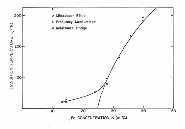
Fig. 29. Magnetic transition temperature vs. iron concentration for the amorphous Fe<sub>x</sub>Pd<sub>80-x</sub>P<sub>20</sub> alloys.
