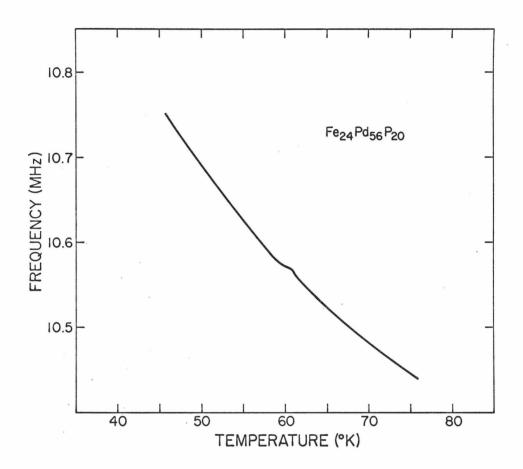
Fig. 27. Frequency measurement for the  $\text{Fe}_{24}\text{Pd}_{56}\text{P}_{20}$ alloy.
