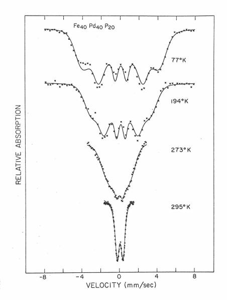
Fig. 21. Temperature dependence of the Mössbauer spectrum for the  $\text{Fe}_{40}\text{Pd}_{40}\text{P}_{20}$  alloy.
