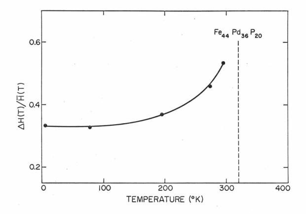
Fig. 35. Temperature dependence of  $\Delta H(T)/\overline{H}(T)$  for the  $Fe_{44}Pd_{36}P_{20}$  alloy. The transition temperature is indicated by the dashed line (320°K).
