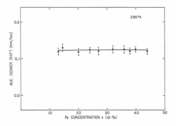
Fig. 6. Isomer shift vs. iron concentration for the amorphous Fe<sub>x</sub>Pd<sub>80-x</sub>P<sub>20</sub> alloys.
