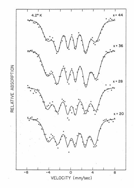
Fig. 31. Illustration of the correlation between isomer shift and hyperfine field described by Eq. (41).
