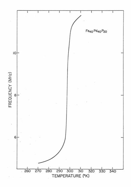
Fig. 25. Frequency measurement for the  $Fe_{40}Pd_{40}P_{20}$  alloy.
