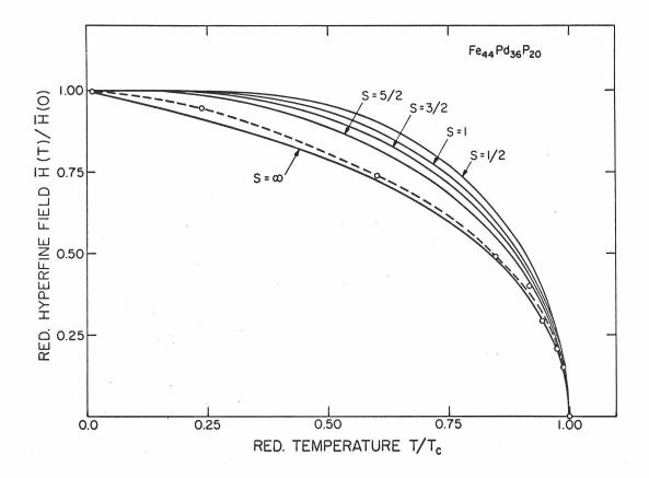
Fig. 33. Reduced (average) hyperfine field vs. temperature for the Fe<sub>44</sub>Pd<sub>36</sub>P<sub>20</sub> alloy (dashed line). The solid curves are the molecular field approximation results for different spin values.
