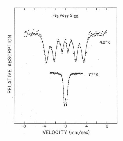
Fig. 32. Mössbauer spectrum of an amorphous Fe<sub>3</sub>Pd<sub>77</sub>Si<sub>20</sub> alloy.
