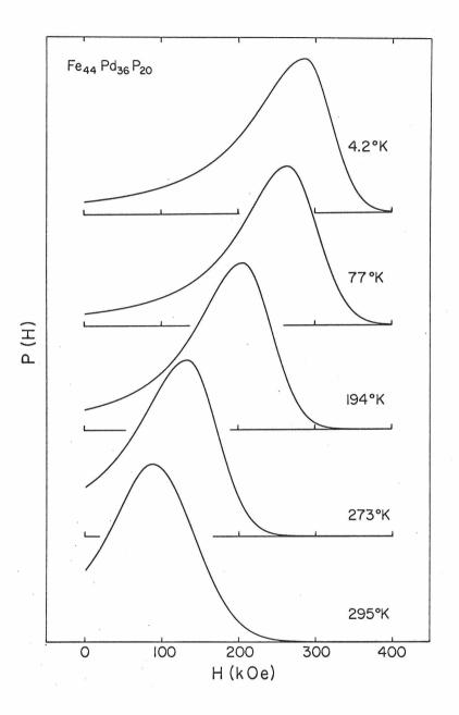
Fig. 19. Temperature dependence of the hyperfine field distribution for the amorphous Fe<sub>44</sub>Pd<sub>36</sub>P<sub>20</sub> alloy.
