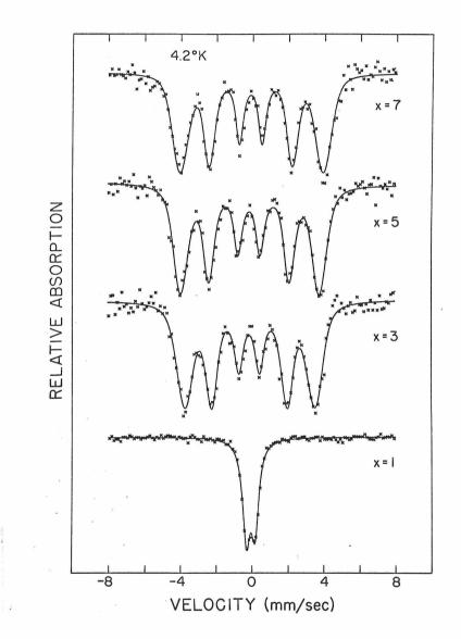
Fig. 39. Mössbauer spectra of amorphous  $\text{Fe}_{x}^{\text{Pd}}$ 80-x<sup>Si</sup>20 alloys at 4.2<sup>°</sup>K.
