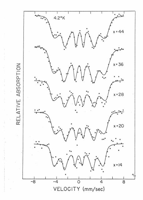
Fig. 11. Mössbauer spectra of the amorphous  $\operatorname{Fe}_{x} \operatorname{Pd}_{80-x} \operatorname{P}_{20}$ alloys at 4.2<sup>°</sup>K. The experimental points are shown and the fitting based on Eq. (32).
