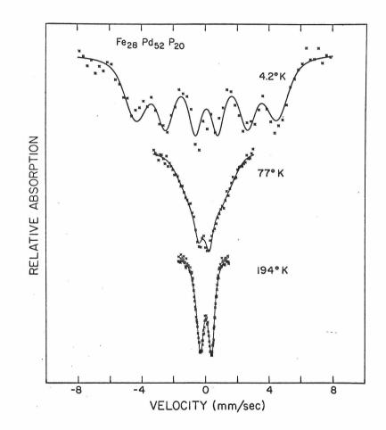
Fig. 24. Temperature dependence of the Mössbauer spectrum for the  $\text{Fe}_{28}\text{Pd}_{52}\text{P}_{20}$  alloy.
