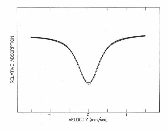
Fig. 17. Illustration of the line broadening caused by the quadrupole interaction in the Mössbauer spectra of the amorphous alloys. The solid curve is the Lorentzian line which best approximates the actual lineshape calculated from Eq. (35).
