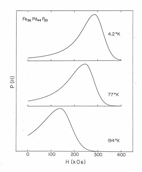
Fig. 23. Temperature dependence of the hyperfine field distribution for the  $Fe_{36}Pd_{44}P_{20}$  alloy.
