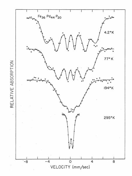
Fig. 22. Temperature dependence of the Mössbauer spectrum for the  $\text{Fe}_{36}\text{Pd}_{44}\text{P}_{20}$  alloy.
