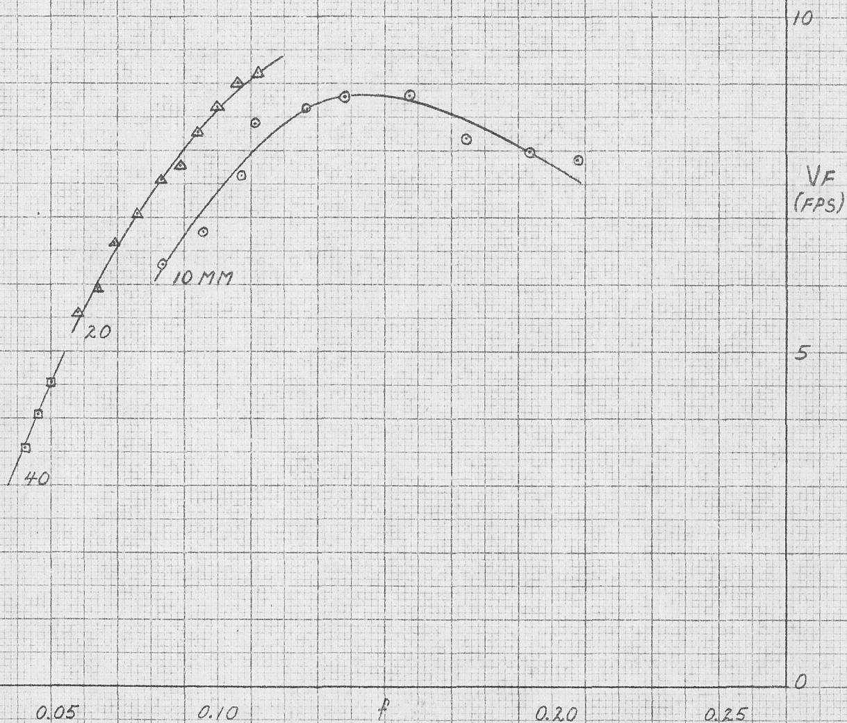
FIG. 10 C_3H_8-O_2 FLAME SPEED DUCT DIA. = 1.25 IN. FLAT FLAME
