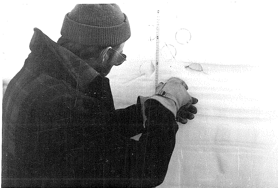
Figure 4d.--Inserting density sample tubes. A thin metal plate was used to push sample tubes beyond the face of the test wall. This makes the lines seen cutting across the circles on the test wall. Samples were placed in an attempt to get representative measurements for individual layers, but sometimes it is impossible to avoid sampling across layer boundaries. The placement of tubes with respect to a hard layer is shown.
