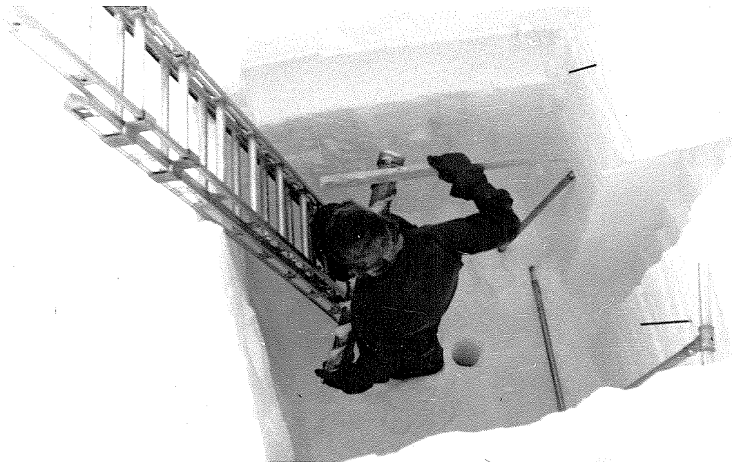
Figure 4f.--Stratigraphic control was extended below the pit floors by core drilling (see p. 10).
