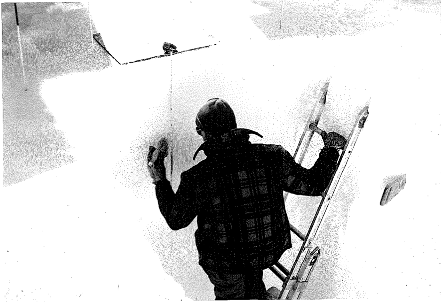
Figure 4a.--Test wall of a pit being brushed to make strata stand out clearly in the upper 6 m where resistance to this "erosion" varies markedly. Note the undisturbed surface at edge of the test wall.
