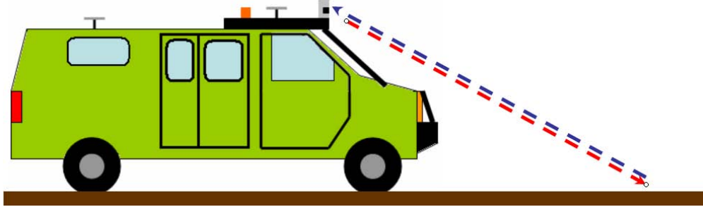
Figure 2.3: A diagram of how LADAR works: a pulse of light is emitted from the LADAR. The light then bounces off an object in the environment, and reflects back to a sensor in the LADAR. The time it takes for the pulse to be emitted and then reflected is used to report the range. This procedure is done dozens of times a second as a mirror within the LADAR spins, allowing measurements to be taken in an arc in the robot’s direction of travel.
