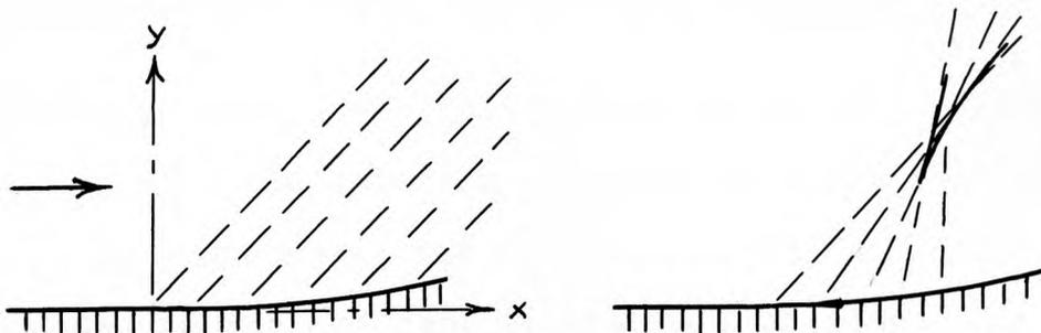
Fig. 2.5. First- and Second-Order Flow Past a Parabolic Bend
