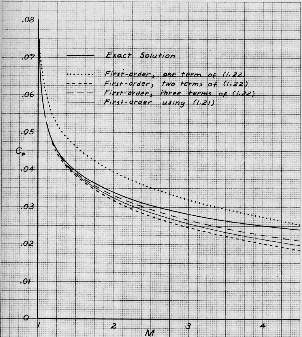
Fig. 1.2. Comparison of First-order Solutions for 5° Cone Using Various Pressure Relations.
