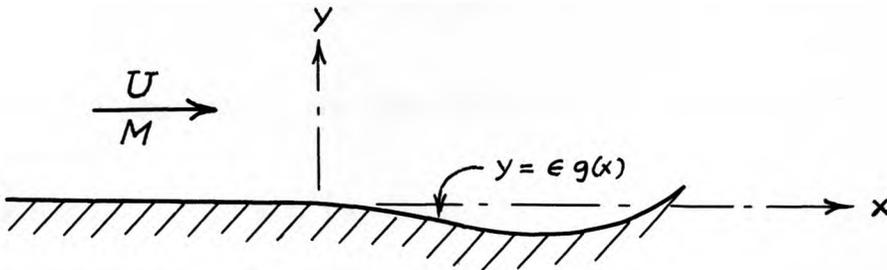
Fig. 2.1. Flow Past a Curved Wall
