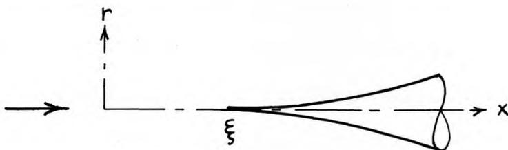
Fig. 3.5. Body Formed by Source Line of Quadratic Strength
