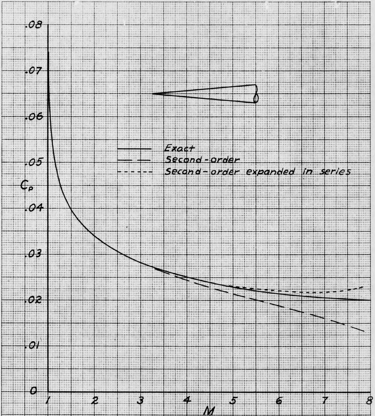
Fig. 2.8. Effect of Expanding in Series upon Second-order Pressure on a Cone.
