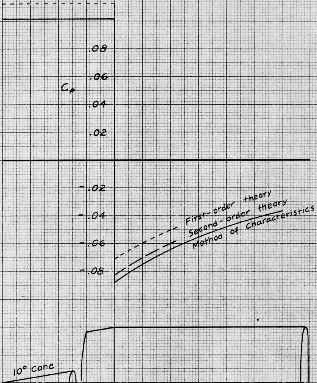
Fig. 3.9. Pressure Distribution on Cone-Cylinder Combination,  $M = 2.075$ .
