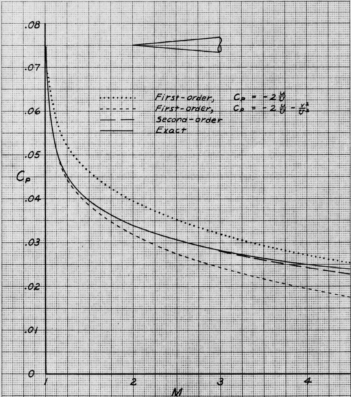
Fig. 2.7. Comparison of Various Approximations for Pressure on a Cone
