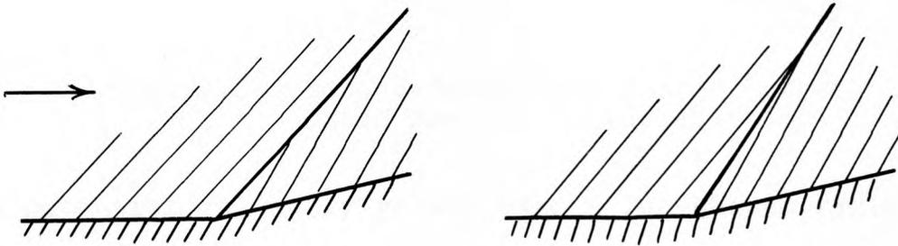
Fig. 2.3. Mach Lines Before and After Adjustment of Potential Discontinuity
