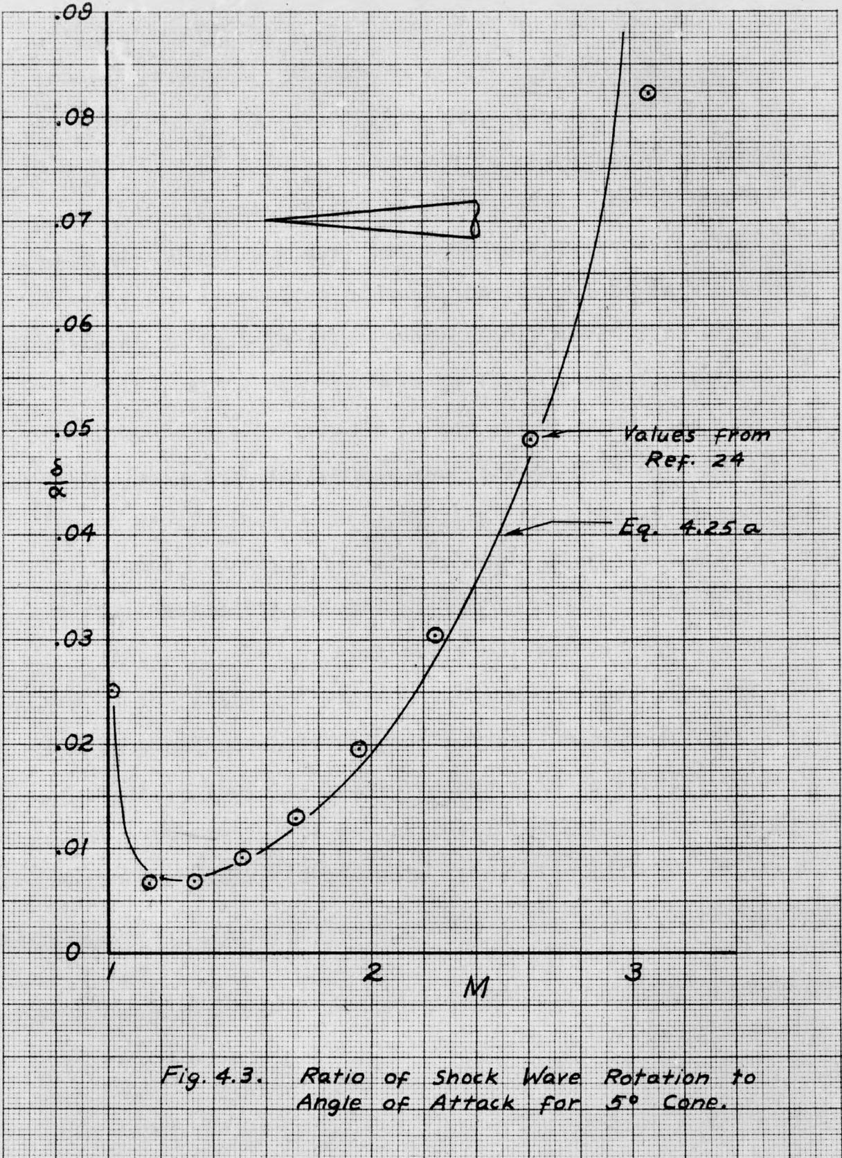
Fig. 4.3. Ratio of Shock Wave Rotation to Angle of Attack for 5° Cone.
