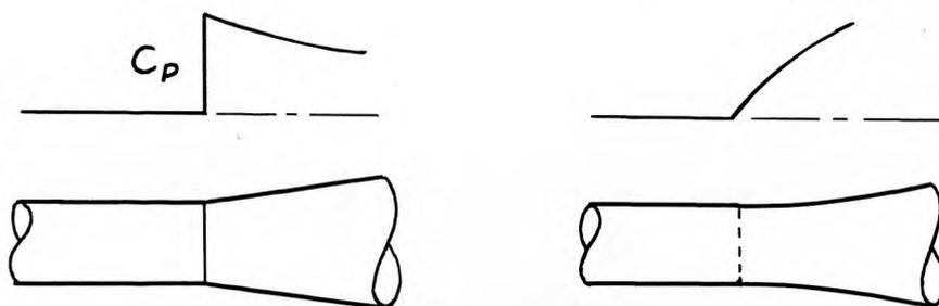
Fig. 3.3. Pressure Distributions Near Discontinuities in Slope and Curvature
