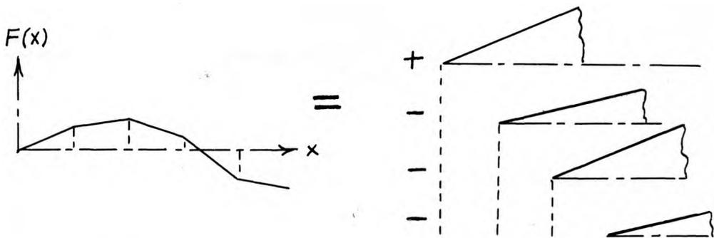
Fig. 3.4. Equivalence of Polygonal Source Strength and Sum of Conical Sources
