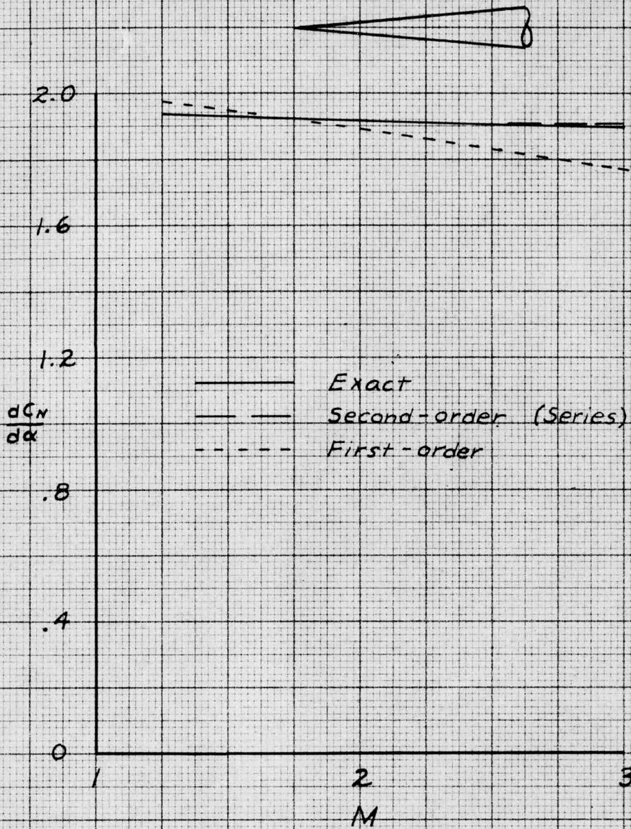
Fig. 4.2. Normal Force Slope for Cone.
