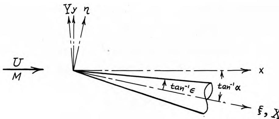
Fig. 4.1. Coordinate Systems for Cone at an Angle
