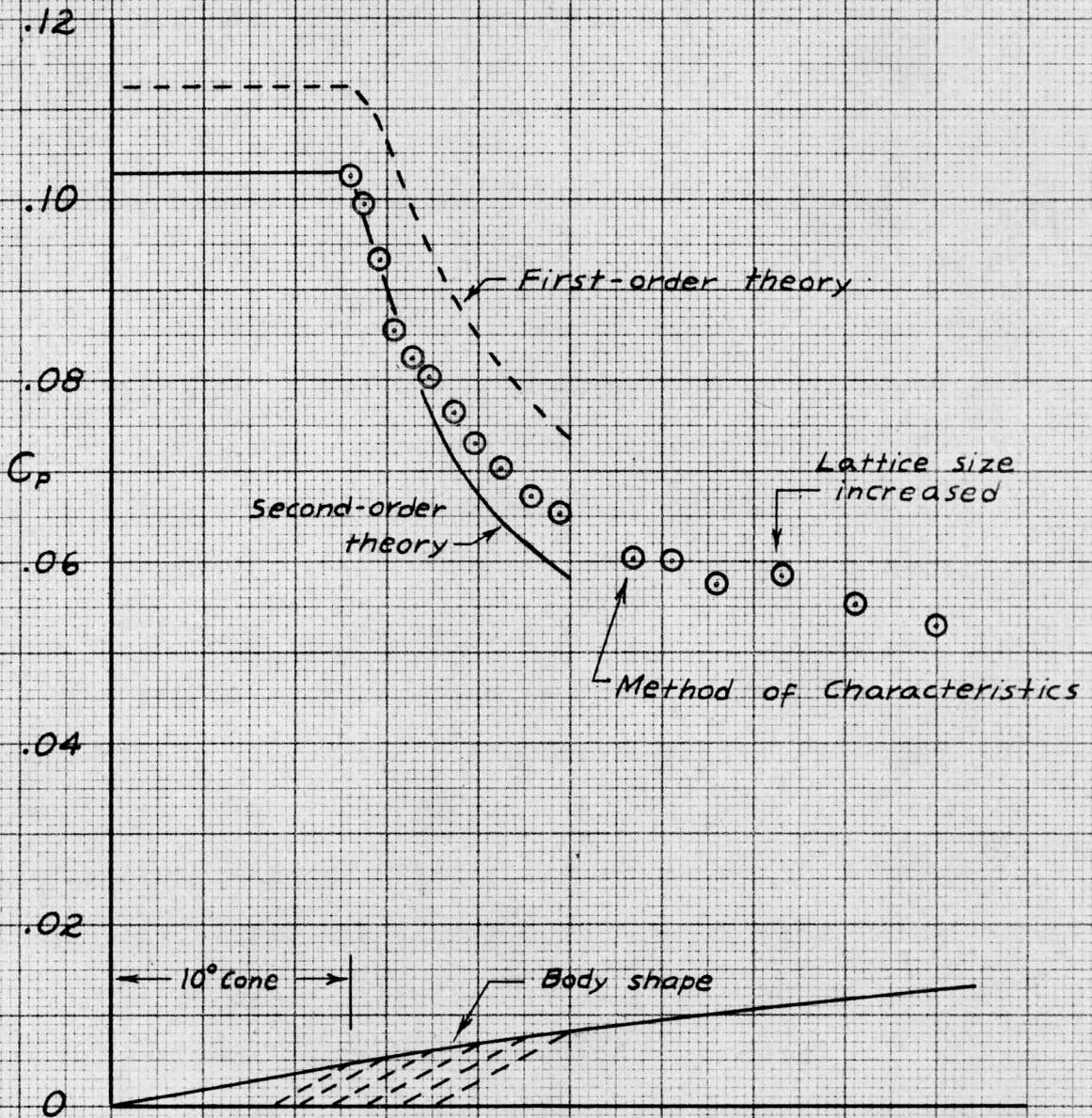
Fig. 3.8. Pressure Distribution on Body of Revolution with Discontinuity in Curvature,  $M = 2.075$
