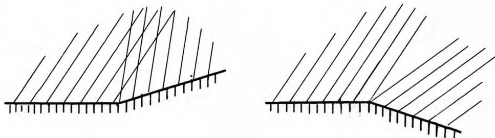
Fig. 2.4. Second-Order Flow Past a Corner Using Revised Characteristics
