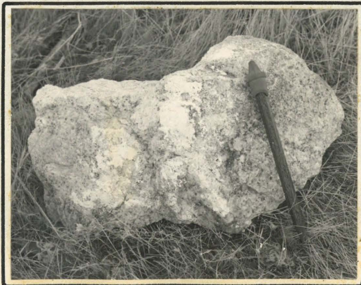
C. Efflorescence on "granodiorite" from Stevenson Creek edit wall
