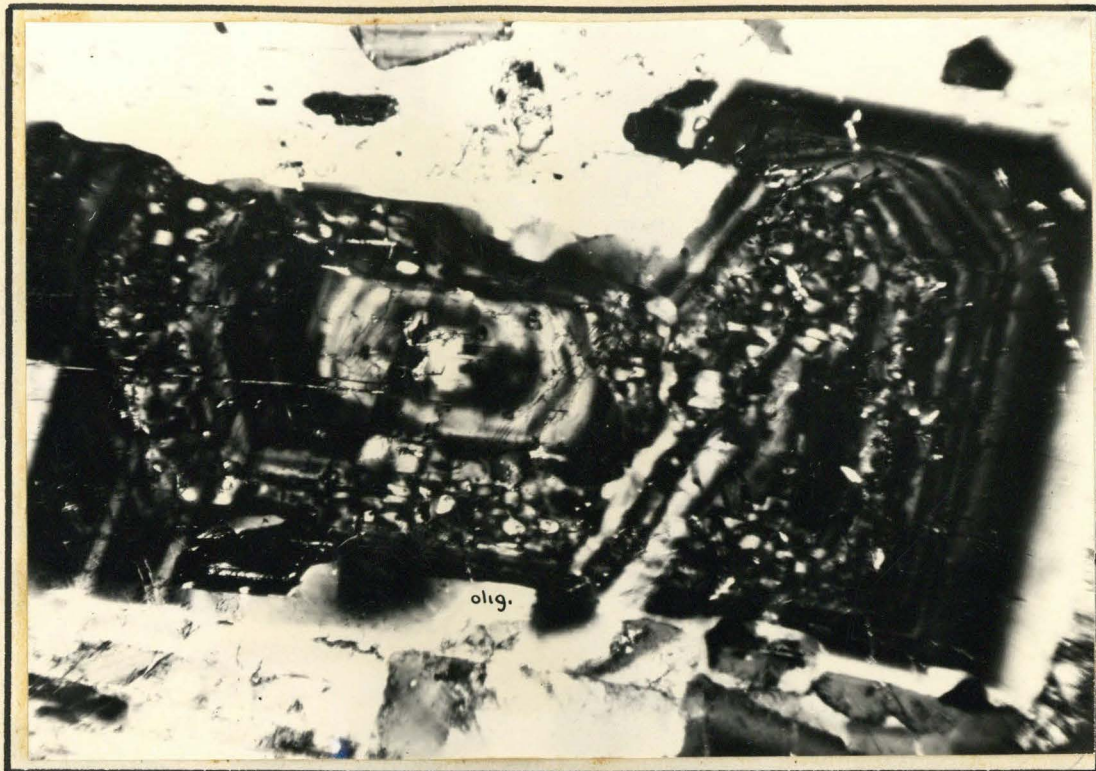
A. Zoned plagioclase crystal, partially replaced by oligoclase 60X Crossed nicols
