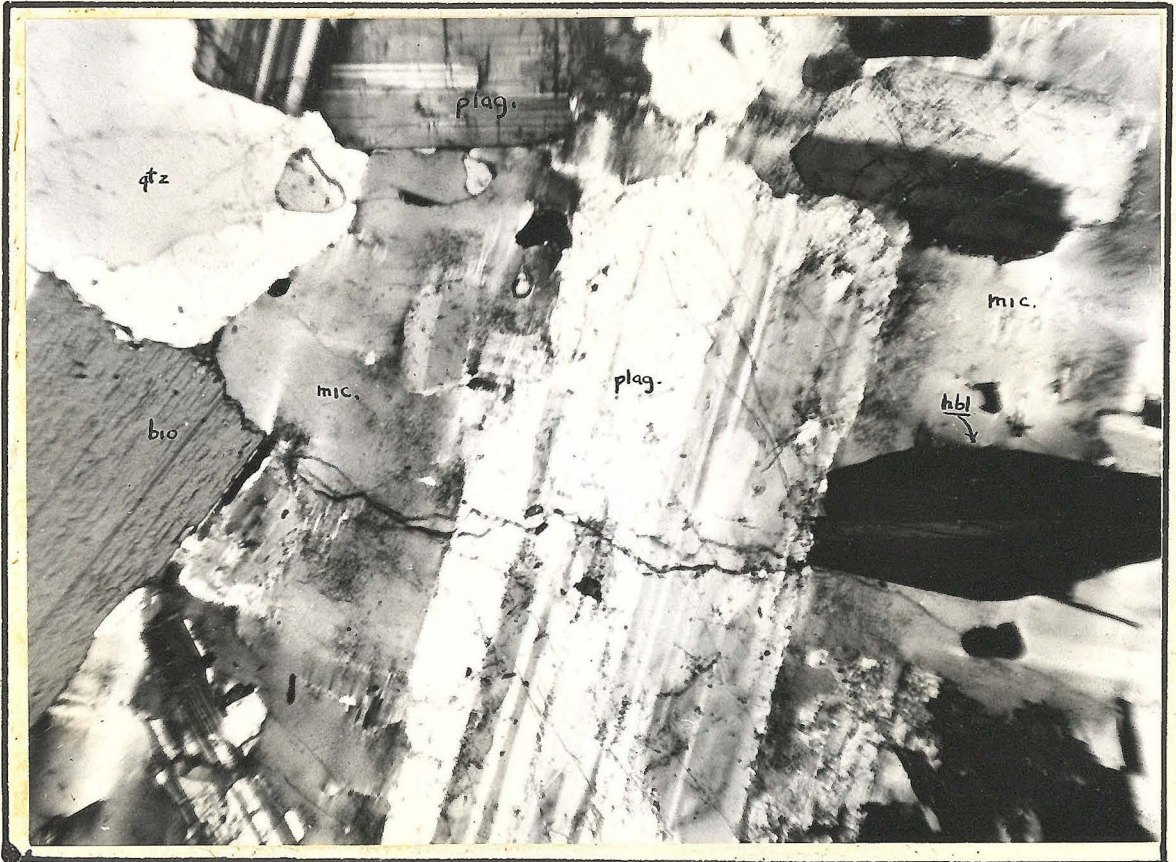
B. Typical "granodiorite" 50x crossed nicols qtz = quartz bio = biotite hbl = hornblende mic = microcline plag = plagioclase
