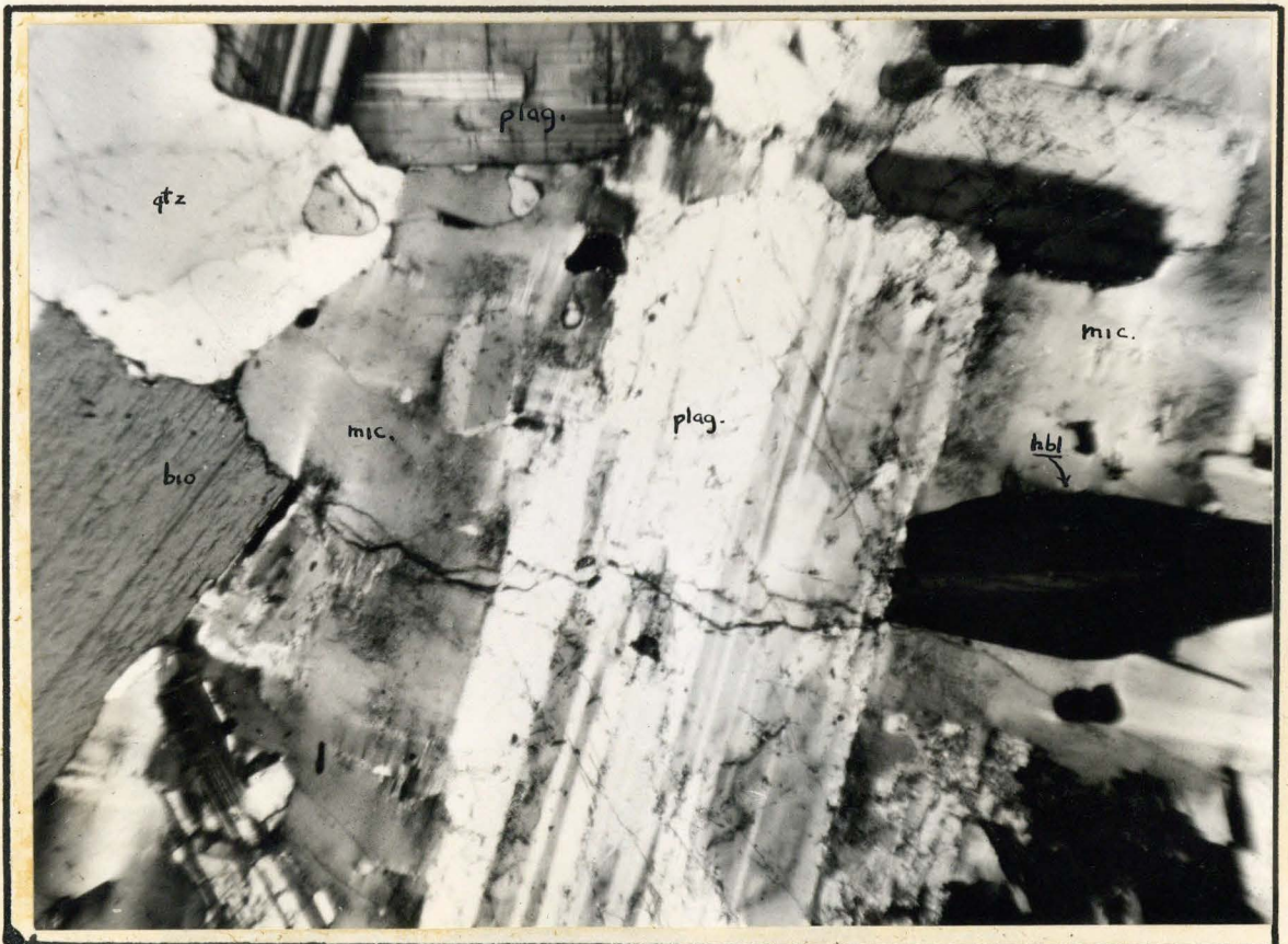
B. Typical "granodiorite" 60X crossed nicols qtz = quartz bio = biotite hbl = hornblende mic = microcline plag = plagioclase
