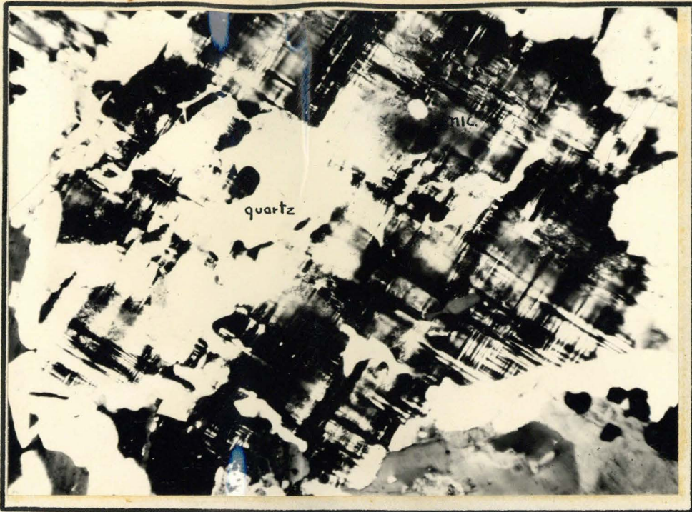
A. Pegmatite - large microcline crystal with inclusions of quartz. 60X Crossed nicols
