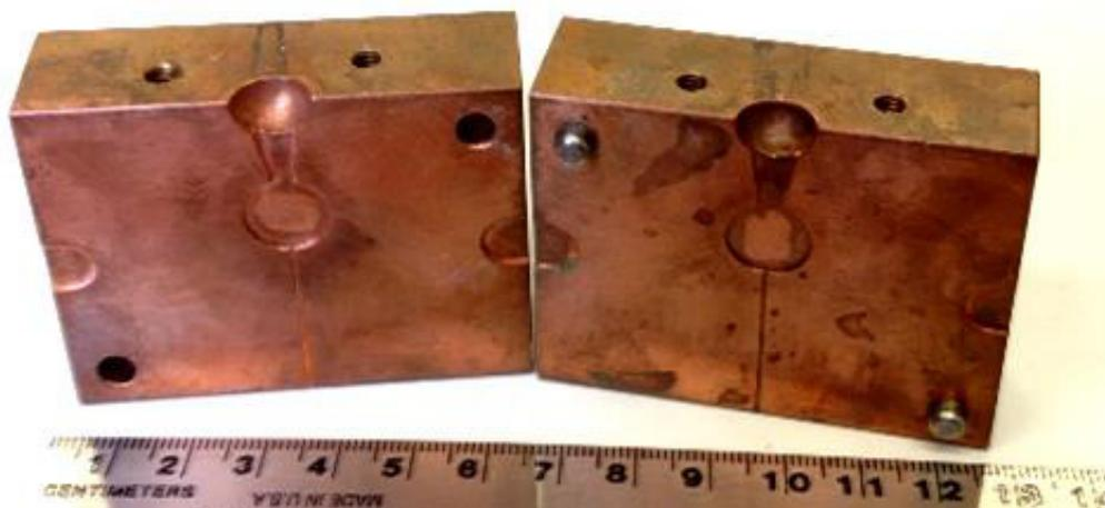
Figure 4.2: Copper mold used to injection mold ferromagnetic metallic glass disks.
