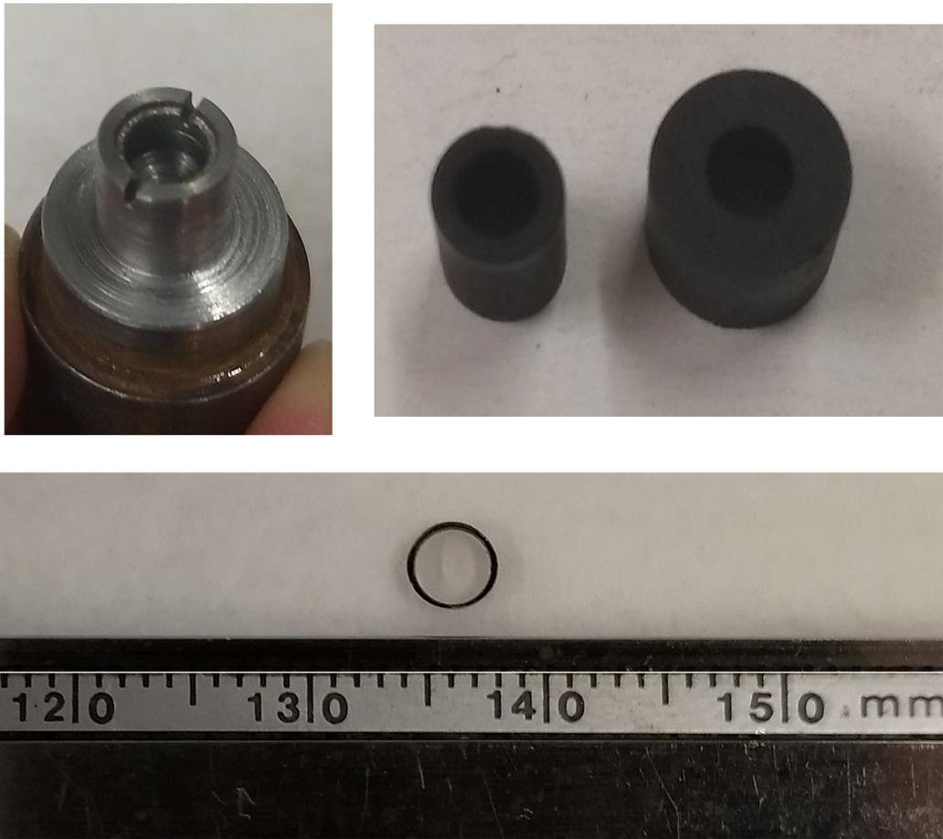
Figure 4.8: EDM holder and cut core. (a) The steel base of the final iteration of holder and the entirety of the first iteration. (b) The graphite top of the final iteration on the sample holder. (c) A cut toroidal core with a wall thickness of 250 microns.
