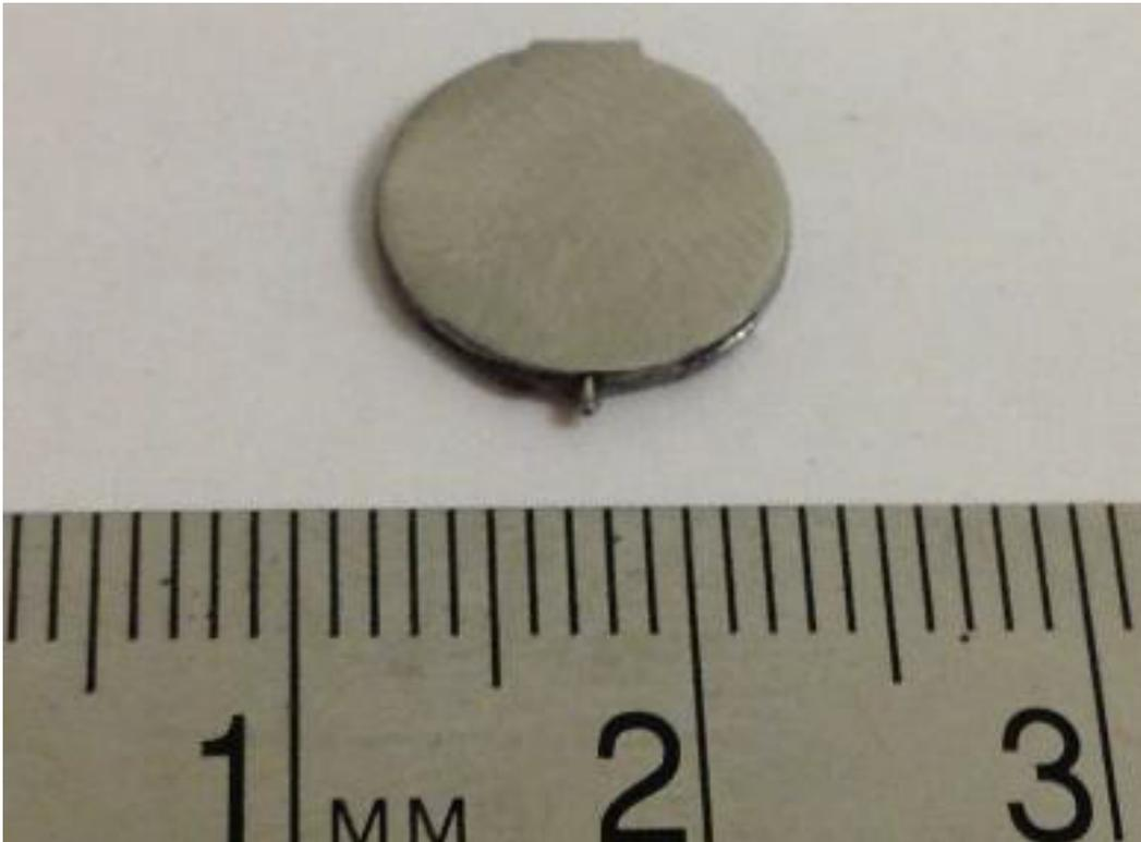
Figure 4.3: Injection cast metallic glass disc of  $\text{Fe}_{68}\text{Mo}_4\text{Ni}_3\text{Co}_5\text{Si}_1\text{B}_{2.5}\text{P}_{11.5}\text{C}_5$ . This sample will then be machined into a toroidal core.
