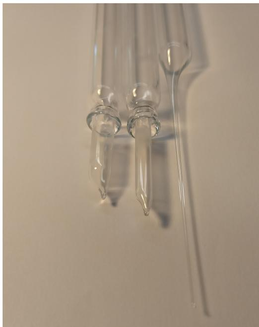
Figure 2.2: A photo of two thin walled quartz tubes with differing diameters, and a quartz capillary.
