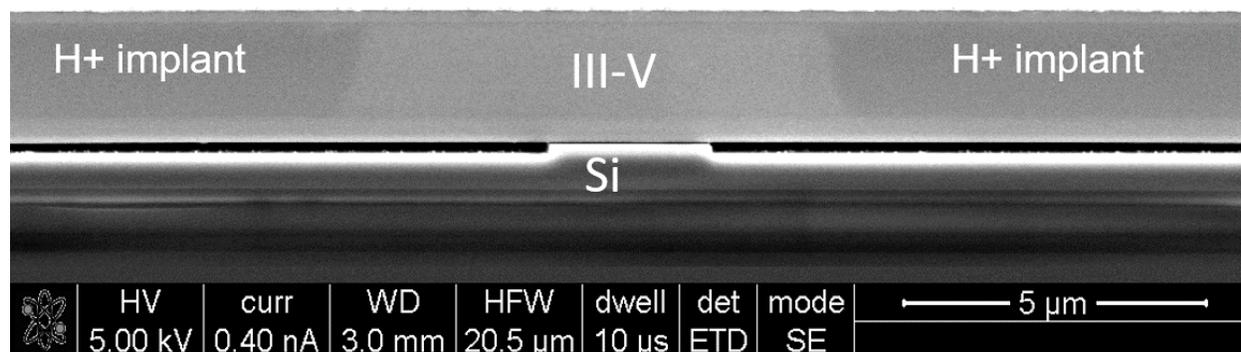
Figure A.18 SEM image of the fabricated laser using ion implantation.
