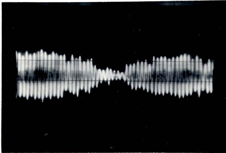
Figure 3.4.9 Oscilloscope trace of the output of channel 2 from the laser-Doppler velocimeter. All beams on; scale: vertical 0.5 V/div., horizontal 0.5 ms/div.
