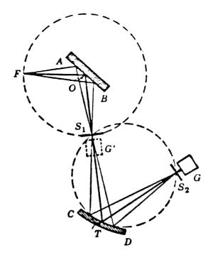
Figure 2.7 Use of crystal monochromator with diffractometer (from Ref. 2.6). A- sample, F- source,  $S_1$ - receiving slit, monochromator,  $S_2$ -detector slit, G- detector.
