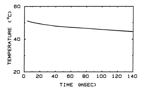
Figure 3.14 Temperature as a function of time during deformation of Ni-Er composite.
