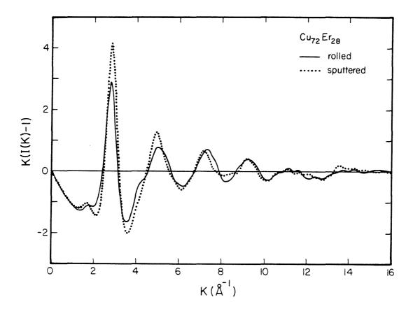
Figure 3.16 Reduced interference function as a function of the magnitude of the K- vector for amorphous  $\text{Cu}_{72}\text{Er}_{28}$  prepared by rolling and sputtering.
