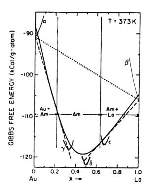
Figure 1.5 Gibbs free energy vs. composition for a mixture of crystalline Au and La (dotted line) and for amorphous  ${\rm Au_XLa_{1-X}}$  alloy (from Ref. 1.11).
