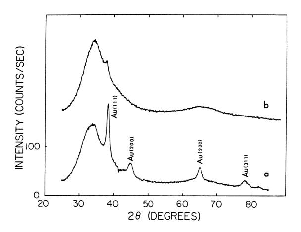
Figure 4.2 X-ray scattering intensity as a function of scattering angle for alternating layers of a-Au $_{34}$ La $_{66}$  and Au: a) as deposited, b) reacted at 80 °C for 4 hr.
