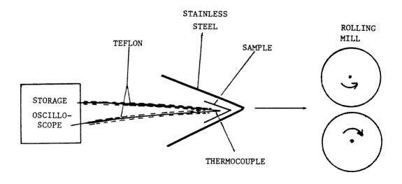
Figure 2.3 Measurement of transient temperature during sample deformation.
