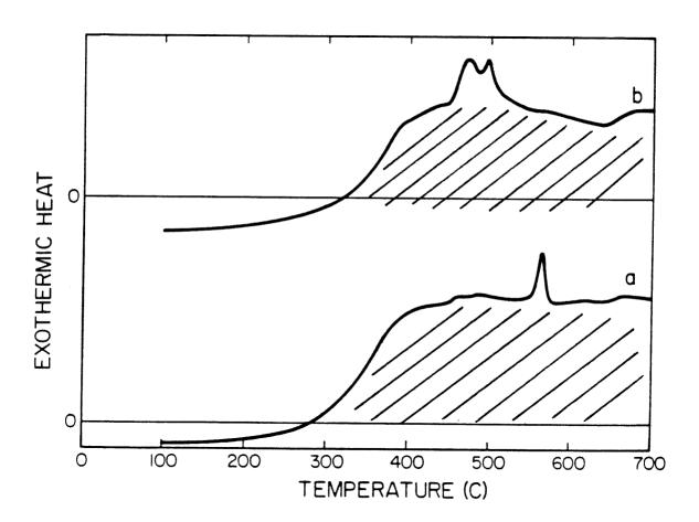
Figure 3.8 DSC scans for  $Cu_{60}Zr_{40}$ , reacted at 275 °C for 8 hr (top) and  $Ni_{68}Zr_{32}$ , reacted at 270 °C for 10 hr, both scanned at a heating rate of 40 °C/min.
