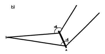
Figure 2.6 X- ray diffraction in reflection (a) vs. transmission (b) geometry.
