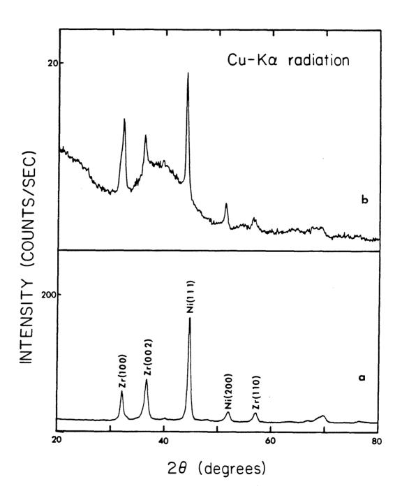
Figure 3.5 X-ray scattering intensity as a function of scattering angle for the samples of Fig. 3.2, measured in transmission geometry.
