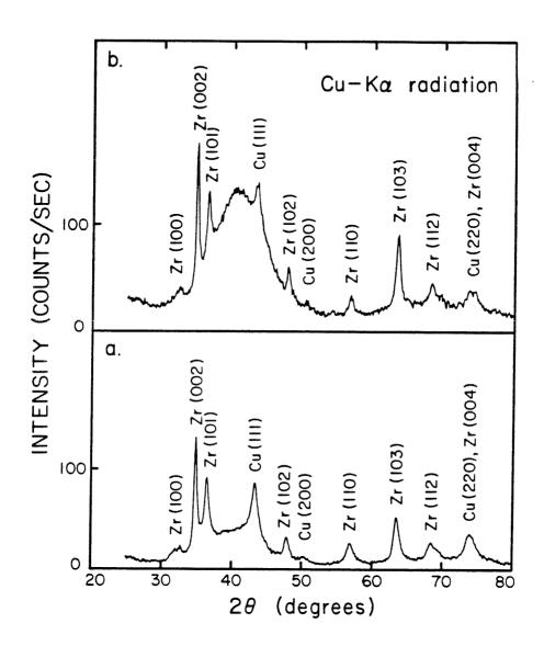
Figure 3.4 X-ray scattering intensity as a function of scattering angle for a  ${\rm Cu_{60}Zr_{40}}$  composite (a) as rolled and (b) reacted at 275 °C for 8 hr.
