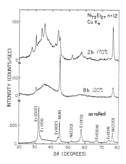
Figure 3.9 X-ray scattering intensity as a function of scattering angle for  $Ni_{73}Er_{27}$  (12 passes) as rolled and reacted.
