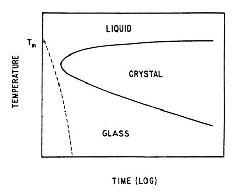
Figure 1.2 Schematic TTT diagram for crystal growth in an undercooled melt (from Ref. 1.7).  $T_{\rm m}$  denotes the melting point.
