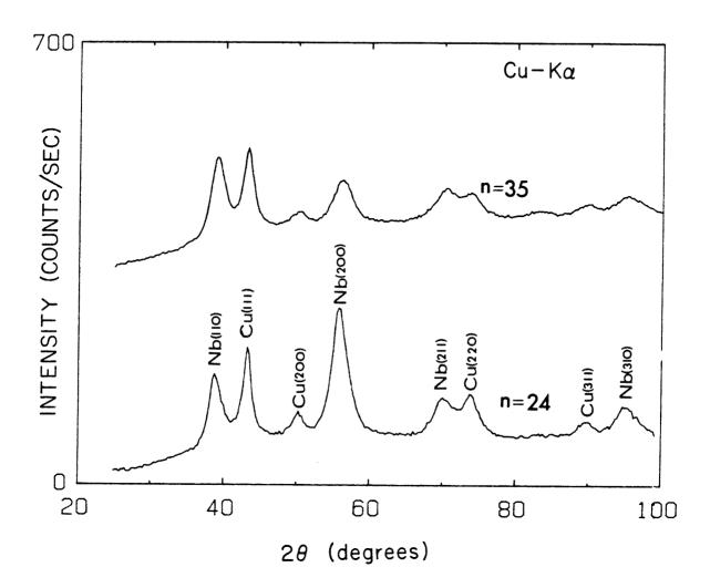
Figure 3.20 X-ray scattering intensity as a function of scattering angle for a crystalline  $\text{Cu}_{75}\text{Nb}_{25}$  composite at different numbers of deformation passes n.
