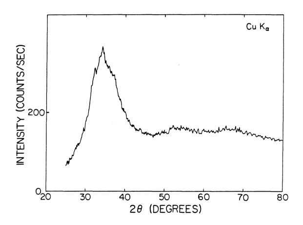
Figure 3.15 X-ray scattering as a function of scattering angle for a  $Cu_{72}Er_{28}$  foil prepared by rapid quenching. Sharp features indicate presence of a small percentage of crystalline material.
