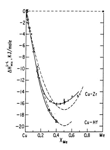
Figure 3.1 Enthalpy of liquid-liquid mixing for copper-zirconium (from Ref. 3.3). The broken line denotes a regular solution fit.
