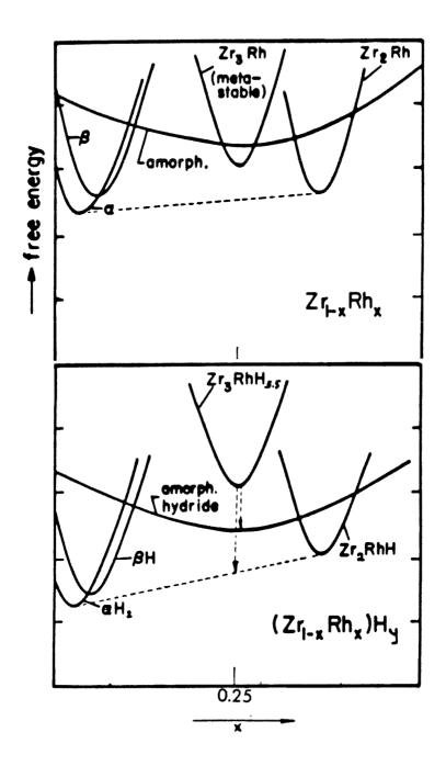
Figure 1.3 Hypothetical free energy diagrams for  $Zr_xRh_{1-x}$  and  $Zr_xRh_{1-x}H_y$  (from Ref. 1.10).
