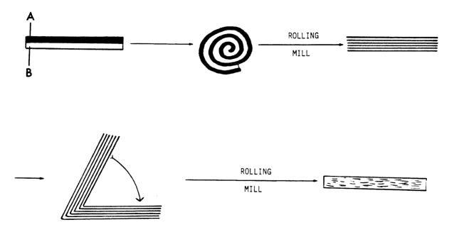
Figure 2.2 Preparation of a composite from elemental foils.
