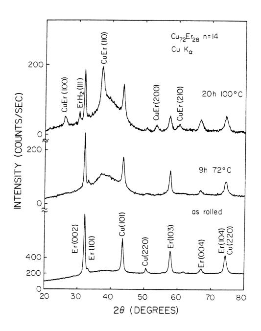
Figure 3.10 X-ray scattering intensity as a function of scattering angle for  $Cu_{72}Er_{28}$  (14 passes) as rolled and reacted.
