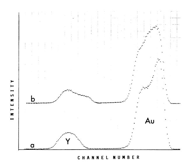
**Figure 4.4** Backscattering of a bilayer of  $Au_{42}Y_{58}$  and Au: a) as deposited, b) reacted at 96 °C for 5.5 hr.
