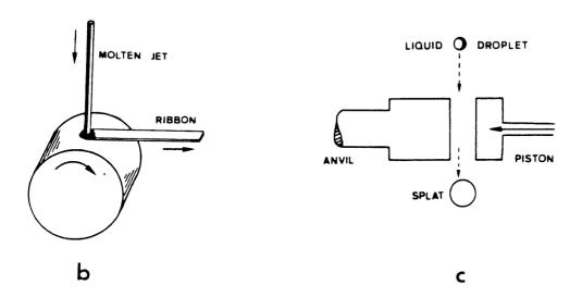
Figure 1.1 Three methods for rapid cooling of liquid alloys, a) "gun", b) meltspinning, c) piston and anvil (from Refs. 1.3,1.4).
