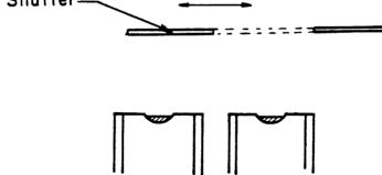
Figure 2.4 Arrangement of Peltier heaters/ coolers in vacuum deposition system (from Ref. 2.3).
