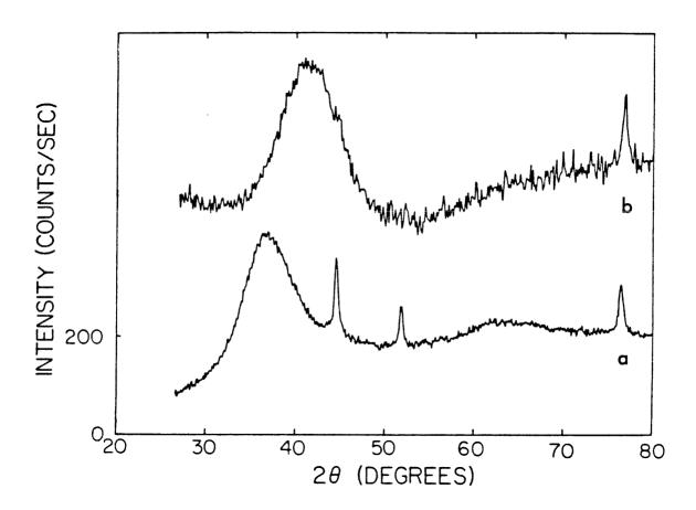
Figure 4.5 X-ray scattering intensity as a function of scattering angle for a composite a- $Zr_2Ni$  - Ni sample with an average composition  $Zr_{52}Ni_{48}$ : a) as rolled, b) reacted for 19 days at 275 °C.
