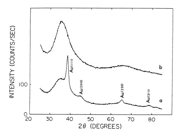
**Figure 4.3** X-ray scattering intensity as a function of scattering angle for alternating layers of a-Au<sub>40</sub>Y<sub>60</sub> and Au: a) as deposited, b) reacted at 102 °C for 5 hr.
