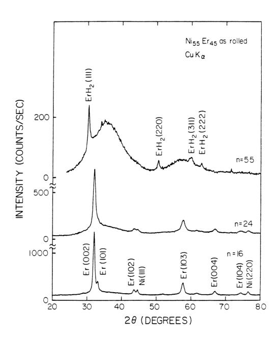
Figure 3.12 X-ray scattering intensity as a function of scattering angle for  $Ni_{55}Er_{45}$  at different numbers of deformation passes n.
