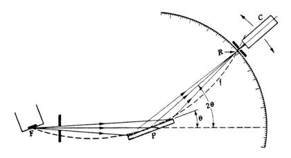
Figure 2.5 X-ray diffractometer in  $\theta$  -  $2\theta$  geometry (from Ref. 2.5). F-source, P- sample, R- receiving slit, C- detector.
