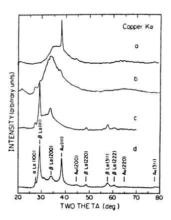
Figure 1.4 X-ray scattering intensity as a function of scattering angle for annealed (4 hr  $\,$  at 80  $^{\rm O}$ C) samples of increasing La content (curves a,b and c) and for an unreacted sample with La content similar to that of curve b (from Ref. 1.11).
