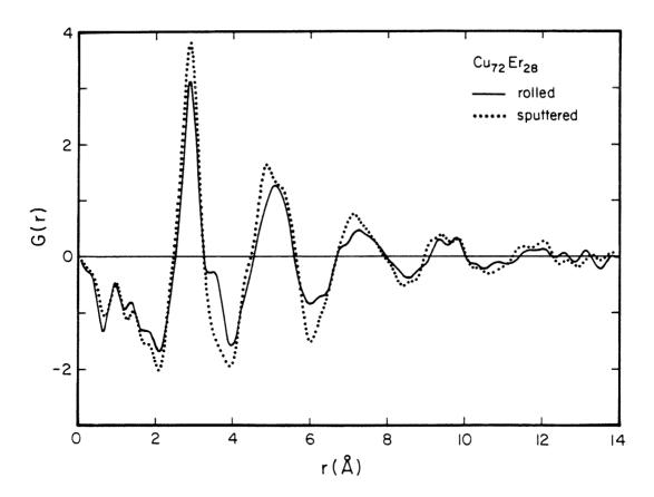
Figure 3.17 Reduced radial distribution functions for amorphous  ${\rm Cu}_{72}{\rm Er}_{28}$  prepared by rolling and sputtering.
