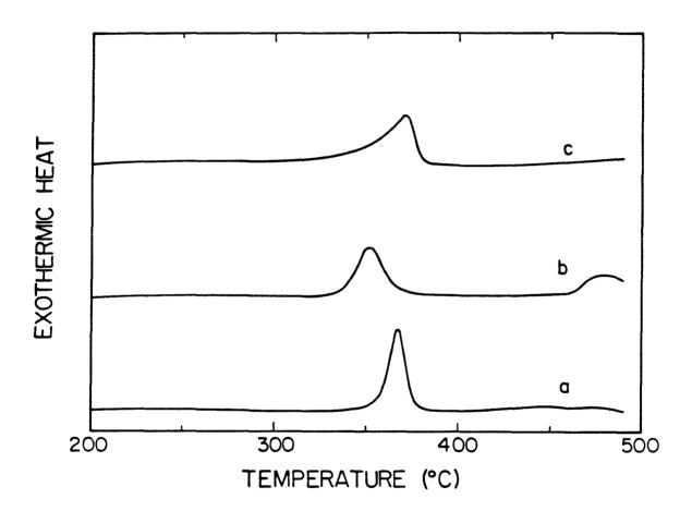
**Figure 3.18** DSC scans at 40 °C/min for amorphous Cu<sub>72</sub>Er<sub>28</sub> prepared by (a) rolling, (b) sputtering, (c) rapid quenching. Sample (c) contains a small percentage of crystals.
