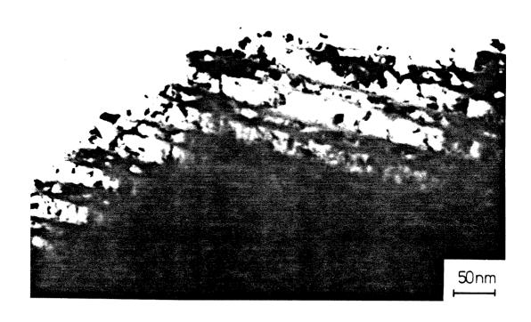
Figure 1.7 Cross- sectional transmission electron micrograph of partially reacted Co-Zr multilayers (from Ref. 1.22).
