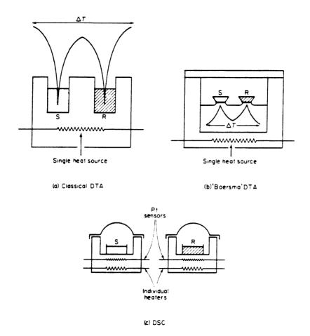
Figure 2.8 Schematic representation of the three principal thermal analysis systems (from Ref. 2.12).
