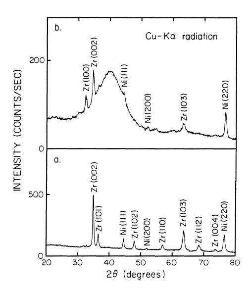
Figure 3.3 X-ray scattering intensity as a function of scattering angle for a  $Ni_{62}Zr_{38}$  composite (a) as rolled and (b) reacted at 260 °C for 14 hr.
