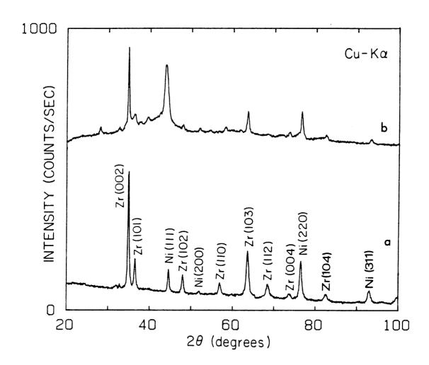
Figure 3.7 X-ray scattering intensity as a function of scattering angle for  $Ni_{62}Zr_{38}$  composite reacted at 340 °C for 4 hr.
