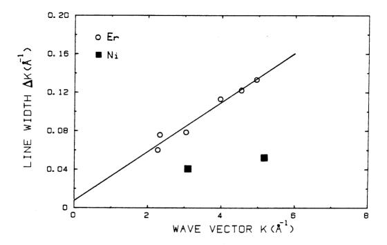
Figure 3.11 Bragg peak broadening  $\Delta K$  as a function of the magnitude of the wave vector for a Ni-Er composite deformed in 12 passes.
