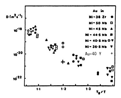
Figure 4.6 Au diffusion coefficients in metal- metal amorphous alloys (from Ref. 4.5). "+" denotes our data point.
