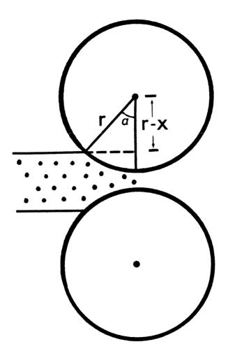
Figure 3.19 Geometry of deformation in a rolling mill.
