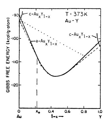
Figure 4.1 Gibbs free energy as a function of composition for the binary system  $\mathrm{Au_XY_{1-X}}$  (from Ref. 4.1). The solid lines denote the amorphous phase and the terminal solid solutions, and the dotted line represents a mixture of a-Au<sub>20</sub>Y<sub>80</sub> with pure gold.
