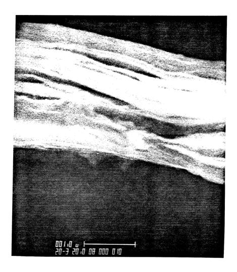
Figure 3.2 Scanning electron micrograph of a cross section of a Ni-Zr composite foil, as rolled.
