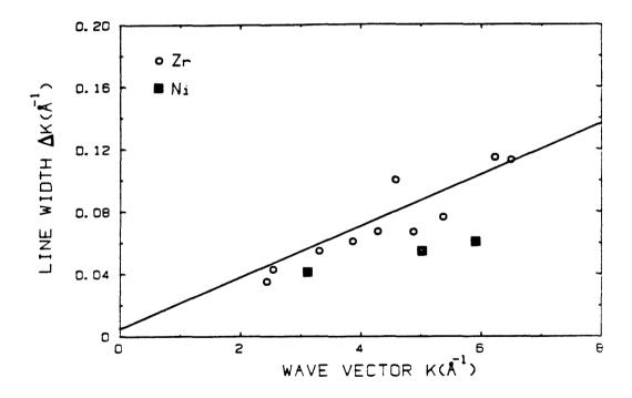
Figure 3.6 Bragg peak broadening  $\Delta K$  as a function of the magnitude of the wave vector for a Ni-Zr composite deformed in 8 passes.
