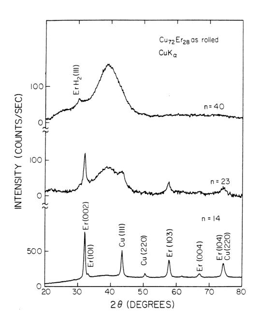
Figure 3.13 X-ray scattering intensity as a function of scattering angle for  $\text{Cu}_{72}\text{Er}_{28}$  at different numbers of deformation passes n.
