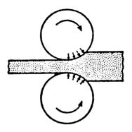
Figure 2.1 Schematic diagram illustrating a rolling mill (from Ref. 2.2).
