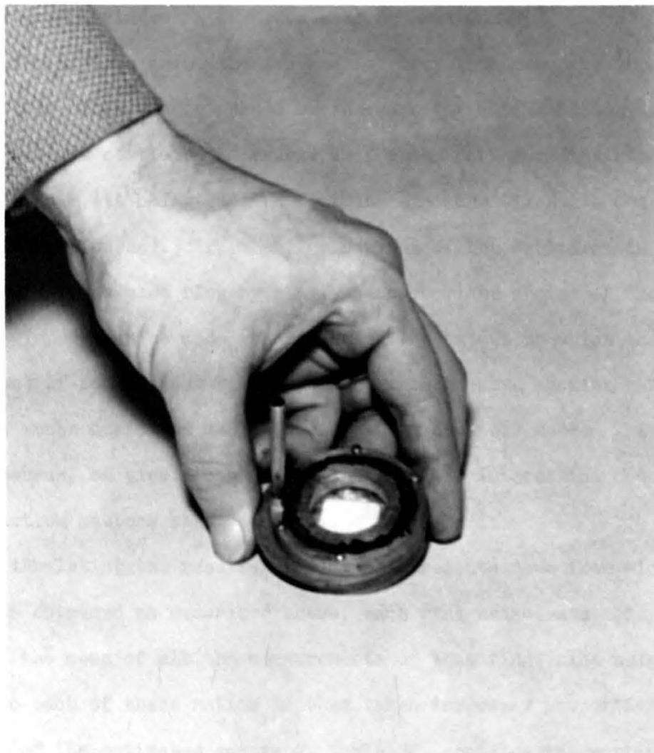
Fig. 13 Photograph of the cell used for the vacuum-air and vacuum-helium experiments.
