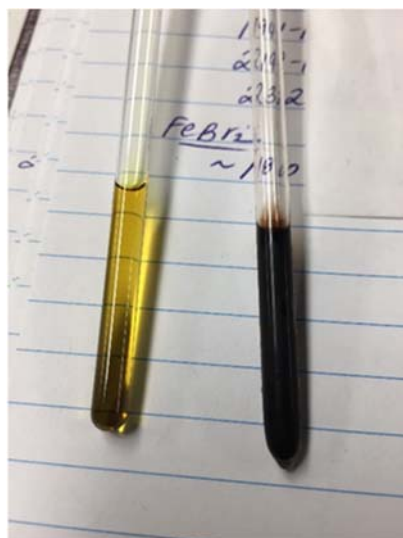
Figure A3.43. Photograph showing qualitative color change of 3.5 pre- (left) and post-photolysis (right).
