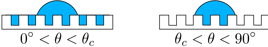
Figure 1.4: Schematic of wetting on a rough, hydrophilic surface.
