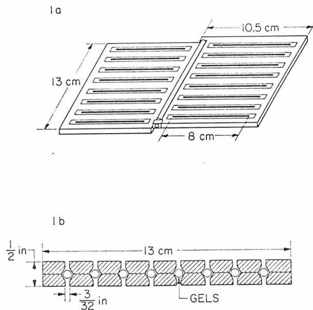
FIG. 1. Destaining rack. (1a) Rack open. It is constructed of two  $\frac{1}{4}$  inch pieces of Plexiglas. The two halves are hinged together by a pin. Eight parallel slots 8 cm long are cut in each sheet of plastic, and the inside edges are then grooved with a  $60^\circ$  included angle mill cutter to  $\frac{1}{2}$  their depth. (1b) Cross-section of closed rack with gels in place.
