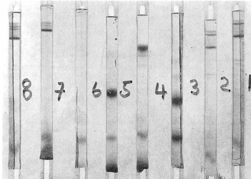
FIG. 3. Destained gels in rack. The samples are partially purified T4 proteins treated with SDS and separated on 5% acrylamide gels with 0.1% SDS (6). They were photographed with fluorescent back lighting using a Wratten 25 filter and Polaroid type 55 P/N film.
