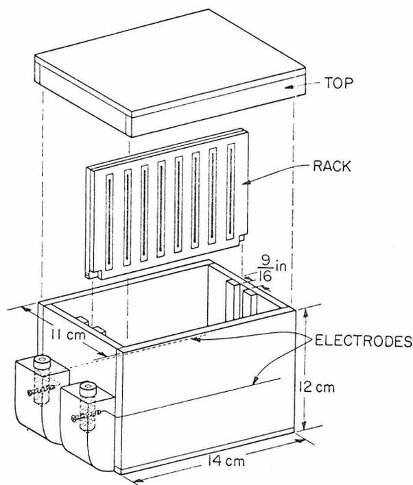
FIG. 2. Complete destainer. The destaining box is made of  $\frac{1}{4}$  inch Plexiglas. The electrodes are platinum wire.
