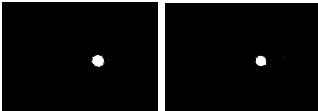
Figure 6.10: The image on the left is the original thresholded image. The one on the right is after a Gaussian blur of size 3 has been passed over the image. Some of the streakier bloom phenomena are removed by the blurring, but the dense bloom region on the right side of the Sun becomes stronger. Because the phenomena is not normally distributed, a Gaussian blur alone does not help improve the performance of the algorithm.
