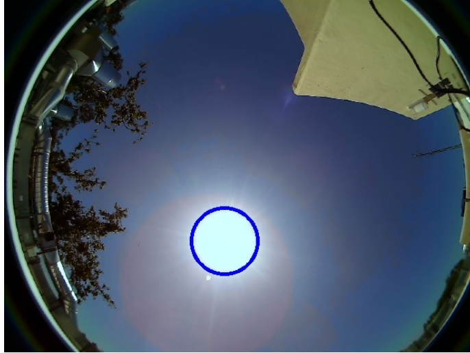
Figure 7.1: The algorithm successfully identifies the Sun while excluding any of the surrounding bloom phenomena. The resulting estimates are within 2^\circ and 3^\circ respectively.
