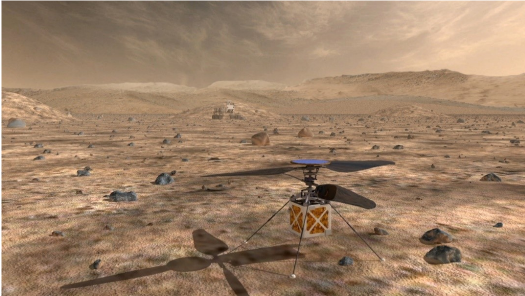
Figure 1.1: Scout, the helicopter that will accompany the Mars 2020 rover. It will be able to explore the region ahead of the rover and communicate back its results and position. (Landau, 2015)
