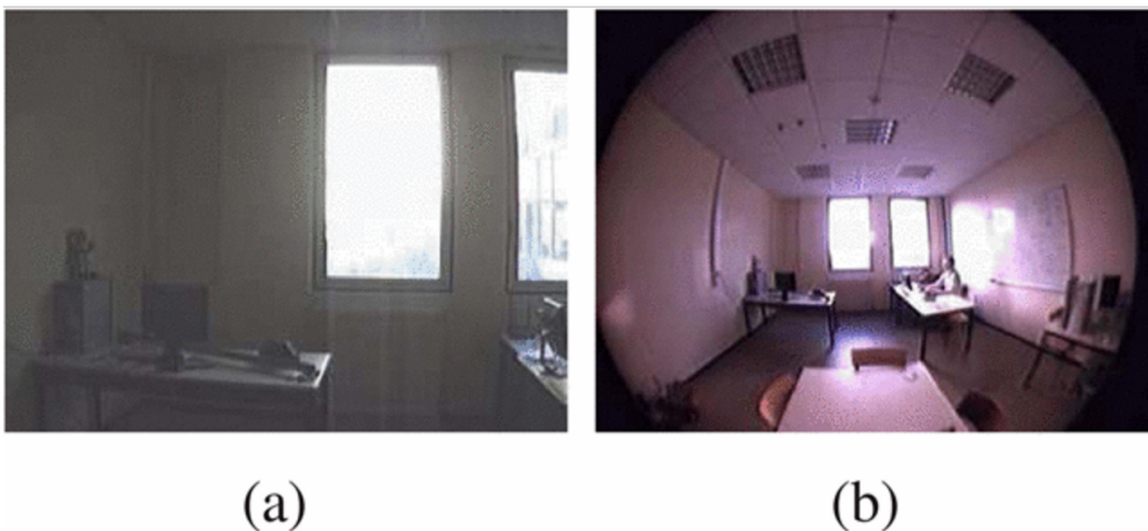
Figure 4.1: An image of a room from a camera with (a) a normal perspective lens and (b) a fisheye lens (Courbon et al., 2007).
