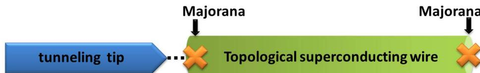
Figure 1.10: One can reveal Majorana zero modes by using tunneling spectroscopy on a topological superconducting wire.
