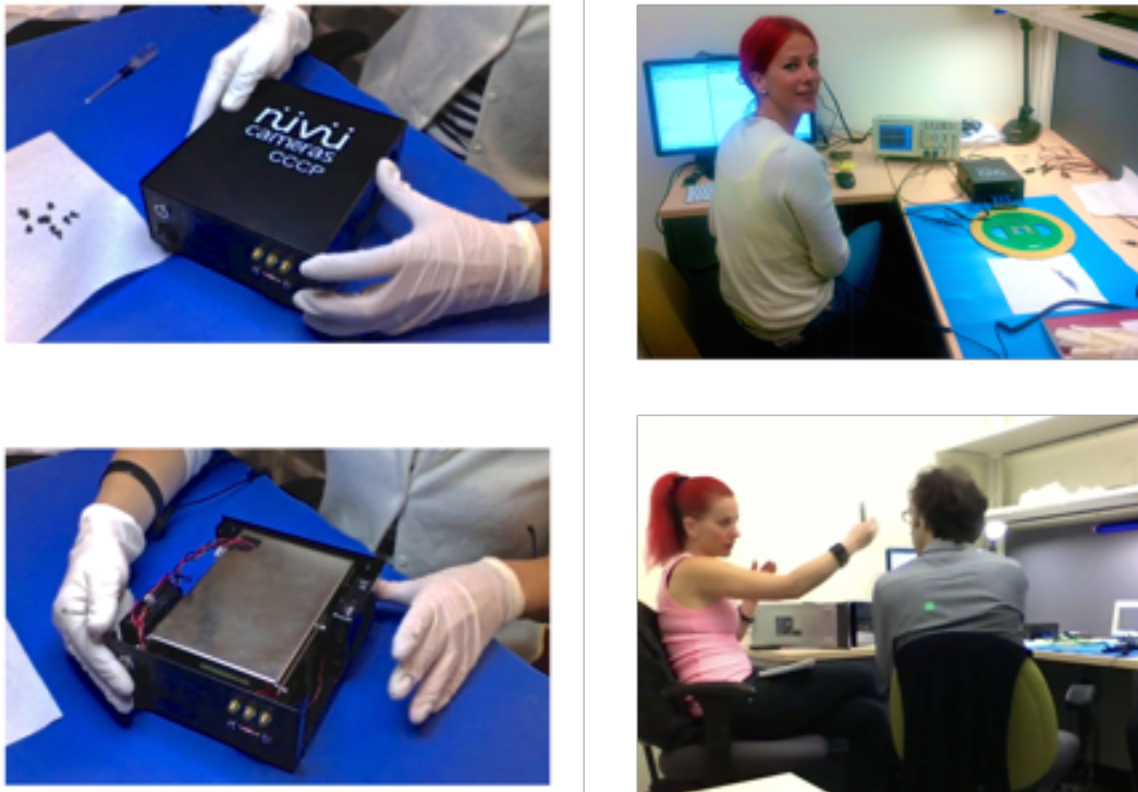
Figure 4.15: Top and bottom left: dual channel CCCP, internal detector boards are not accessible, due to a permanent ribbon cable on the side. Top and bottom right: visit with Olivier Daigle at his lab in Montreal to test my camera system end-to-end (controller, computer, chip, and PCB).
