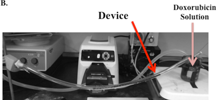
Supplementary Figure 25. A. Doxorubicin clearance from porcine blood in closed loop flow model. B. Closed loop flow model design with 25 magnet device within the lumen of the flow model.
