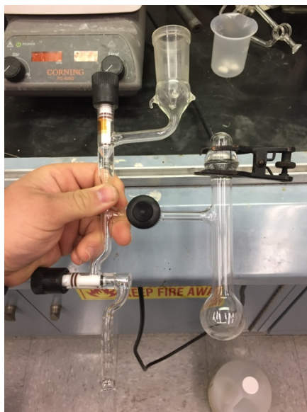
Figure 4.13. Custom laser cell for STOIR-O 2 experiments. Design allows the introduction of macroscopic carbon fiber electrodes while maintaining an oxygen-free atmosphere.
