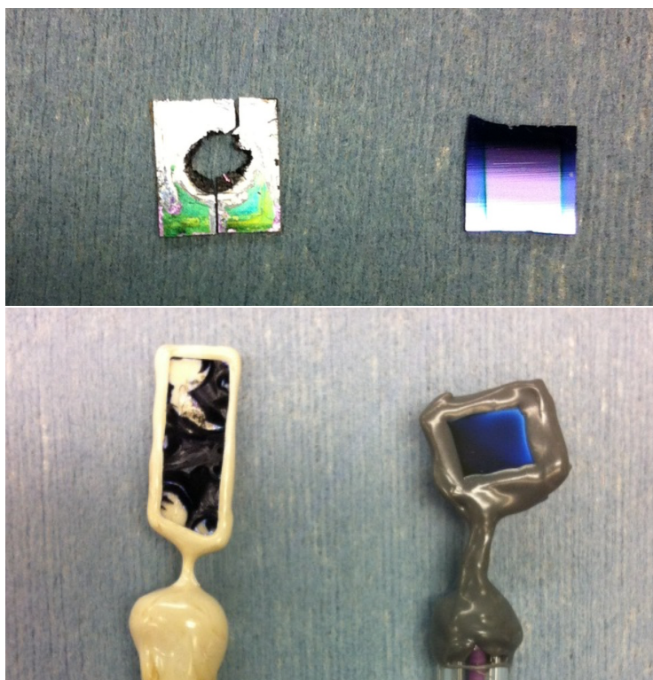
Figure 1.4: Corrosion of GaAs in 1.0 M KOH(aq) using a compression cell (top) and epoxied electrode (bottom) with and without an ALD- \text{TiO}_2 protection layer.
