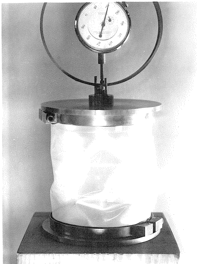
Fig. 7 Photograph of Buckled Mylar Cylinder with 1-1/2-inch Spaced Free, Protruding-in Plexiglass Ring-Stiffeners.
