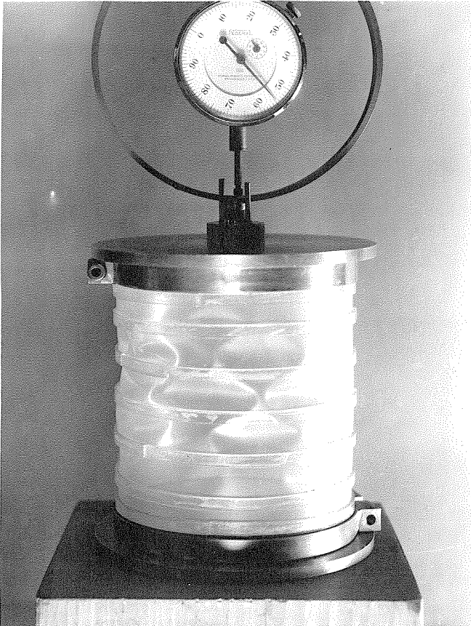
Fig. 6 Photograph of Buckled Mylar Cylinder with 5/8-inch Spaced Fixed, Flat Unbroken Plexiglass Ring-Stiffeners.
