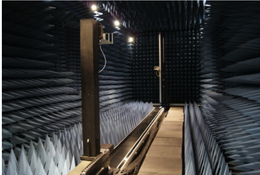
Figure 3.5: Example of a far-field measurement setup in anechoic chamber.
