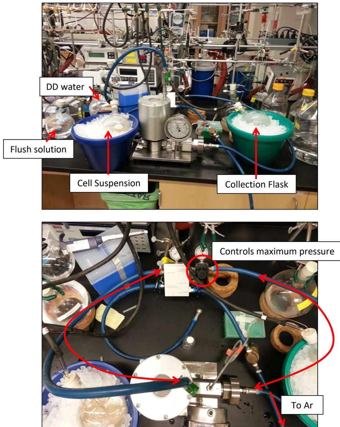
**Figure II-7.** Setup of cell lysis via the EmulsiFlex C5.
