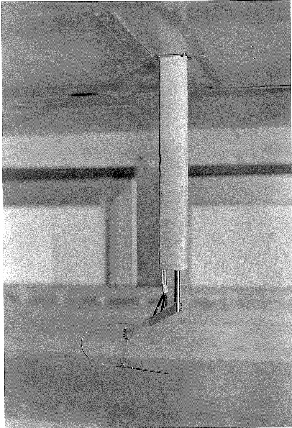
Figure 2.4. Probe mounted on streamlined support.
