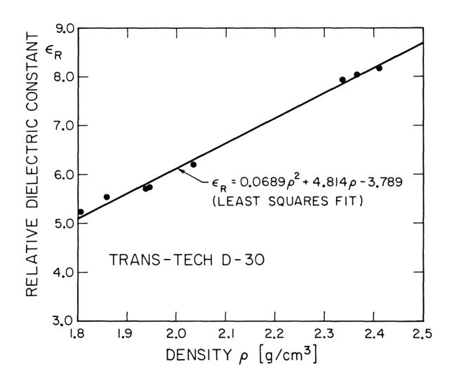
Figure I-7: Relative dielectric constant versus density for Trans-Tech D-30 powder. 70% of particles between 100  $\mu m$  and 43  $\mu m$ , 30% less than 43  $\mu m$ .
