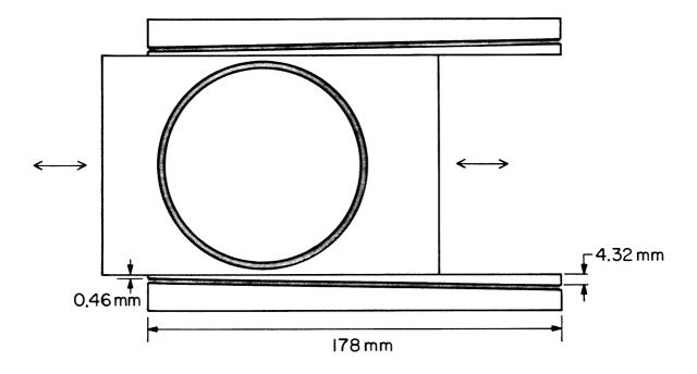
Figure III-2: Coupling scheme used to achieve adjustable distances between a ring resonator and two straight waveguides
