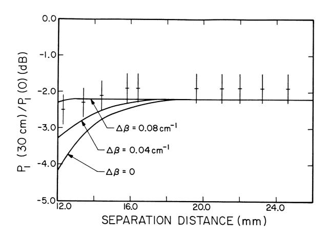
Figure IV-17: Power transmitted to the far end of the primary channel guide (relative to that coupled onto the near end) versus separation distance. The solid curves are theoretical results. The measured points have corrected for the 1 dB loss of the Stycast rods
