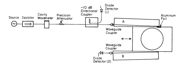
Figure III-3: Set-up for measuring Q's of ring resonators
