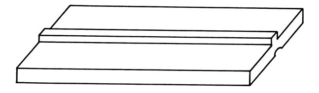
Figure II-5: Die used to emboss grooves in polypropylene
