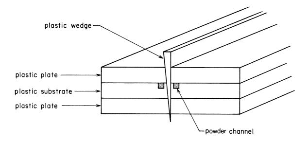
Figure IV-3: Method of achieving variable spacing between two parallel channel waveguides
