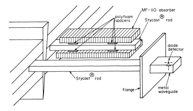
Figure IV-4: Space-saving scheme for terminating one channel guide in a matched load while measuring the power transmitted to the end of the adjacent guide
