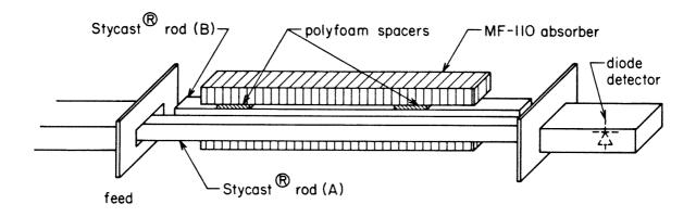
Figure IV-12: Setup for measuring the power transferred between the rod (A) to be used to couple power onto the near end of the primary channel guide and the assembly of the rod (B) and absorbers forming a matched load for the near end of the secondary guide.
