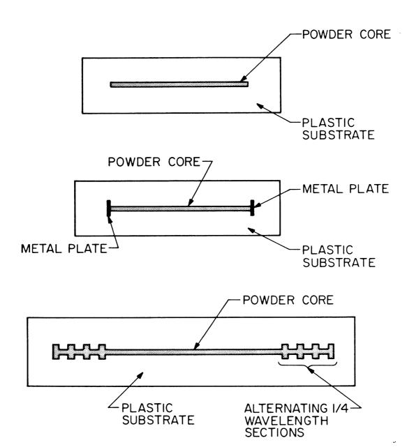
Figure III-1: (a) Segment of straight dielectric channel waveguide
