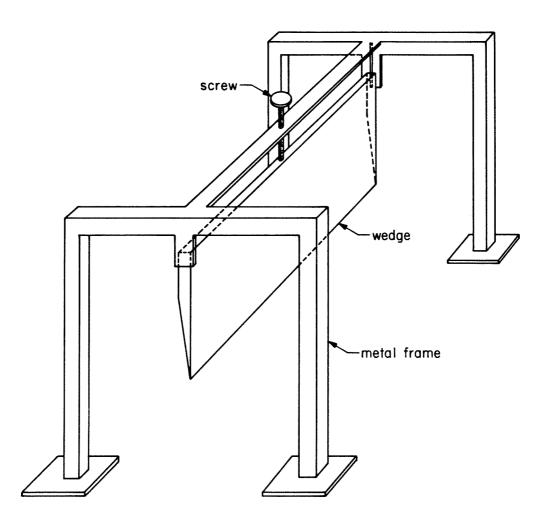
Figure IV-6: Metal frame used to support and guide the  $\ensuremath{\mathsf{Rexolite}}^R$  wedge
