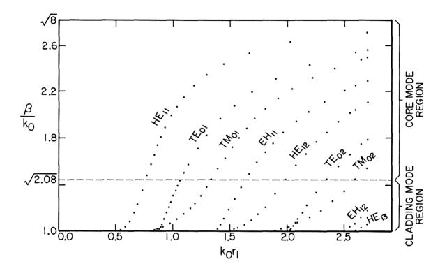
Figure I-4: Dispersion curves of 3-region cylindrical dielectric waveguide.  $\epsilon_{r1}$  = 8,  $\epsilon_{r2}$  = 2.08,  $\epsilon_{r3}$  = 1.  $r_2$  = 1.25  $r_1$ .
