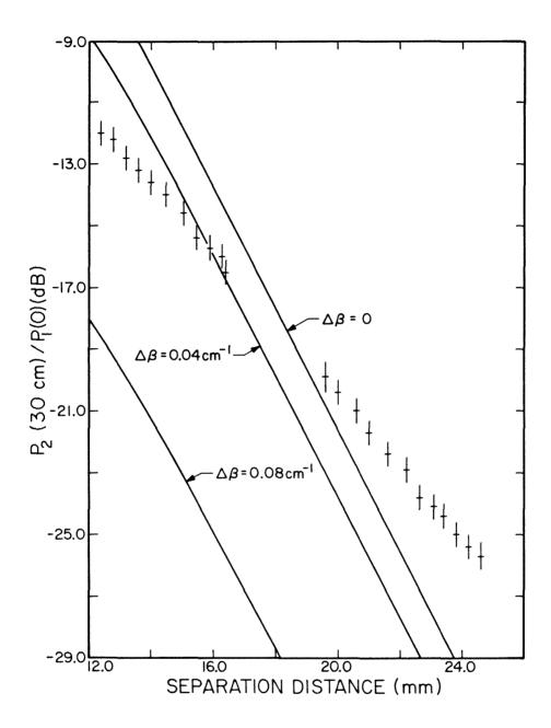
Figure IV-18: Power transmitted to the far end of the secondary channel guide (relative to that coupled onto the near end of the primary guide) versus separation distance. The solid curves are theoretical results. The measured points have been corrected for the 1 dB loss of the Stycast rods.
