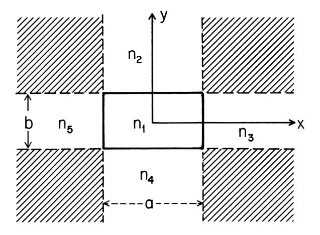
Figure II-2: Cross section of dielectric waveguide analyzed by Marcatili
