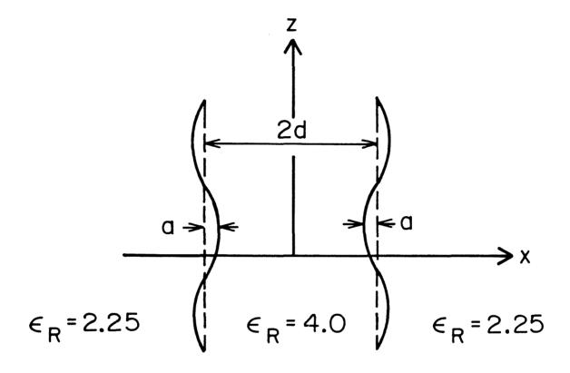
Figure AIV-2: Longitudinal cross section of a dielectric slab with sinusoidal thickness variation
