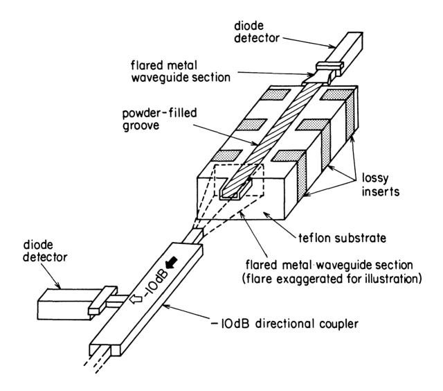
Figure II-3: Setup for measuring attenuation and guide wavelength
