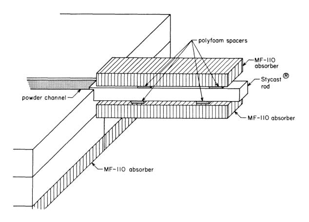
Figure IV-11: Matched termination for a channel guide
