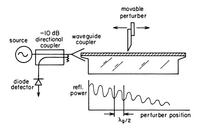
Figure II-4: Guide wavelength measurement
