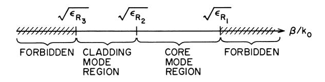
Figure I-2: Core mode and cladding mode regions of a 3-region cylindrical dielectric waveguide
