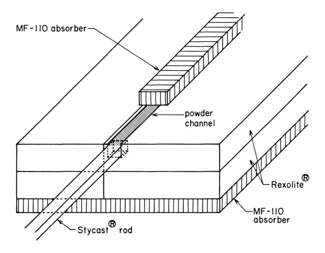
Figure IV-10: Setup for testing coupling between a  $\operatorname{Stycast}^R$  rod and a channel guide
