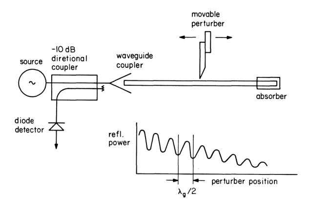
Figure I-8: Schematic of setup for guide wavelength measurement.
