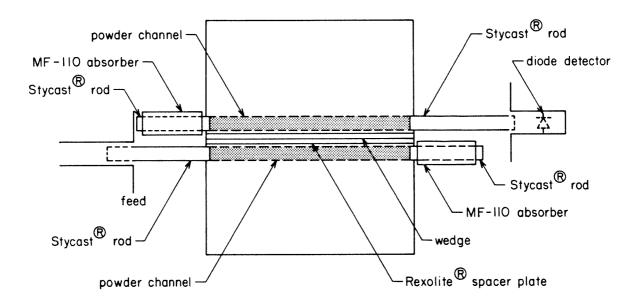
Figure IV-15: Top view schematic of setup for testing the channel guide directional coupler
