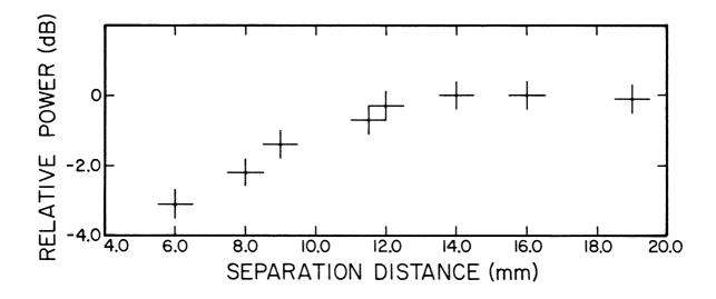
Figure IV-13: Power detected at the far end of the rod A relative to the amount detected in the absence of rod B and its accompanying absorbers
