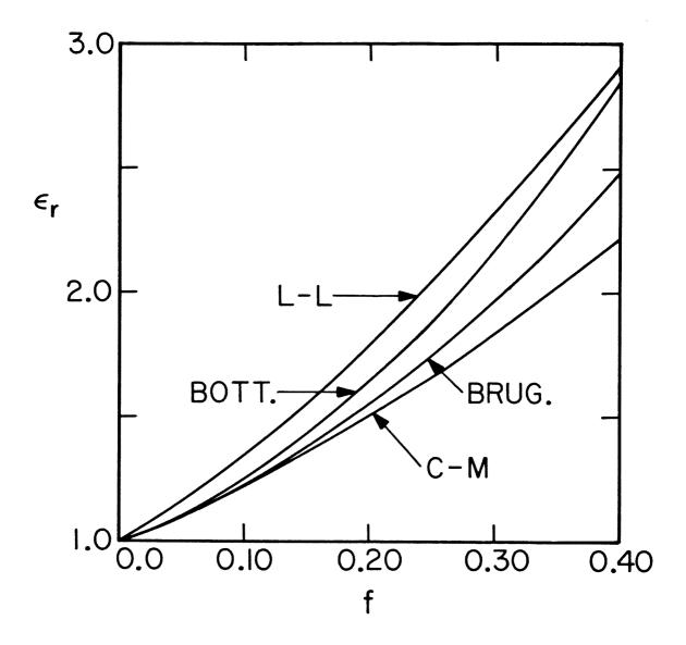
Figure AII-1: Theoretical curves of power effective dielectric constant versus volume fraction for particles composed of a material with a dielectric constant of 9.0 (A1<sub>2</sub> O<sub>3</sub>). The formulas of Clausius and Mossoti, Bottcher, Bruggemann, and Looyenga for spherical particles are each represented.
