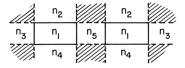
Figure IV-2: Cross-section of the directional coupler analyzed by Marcatili
