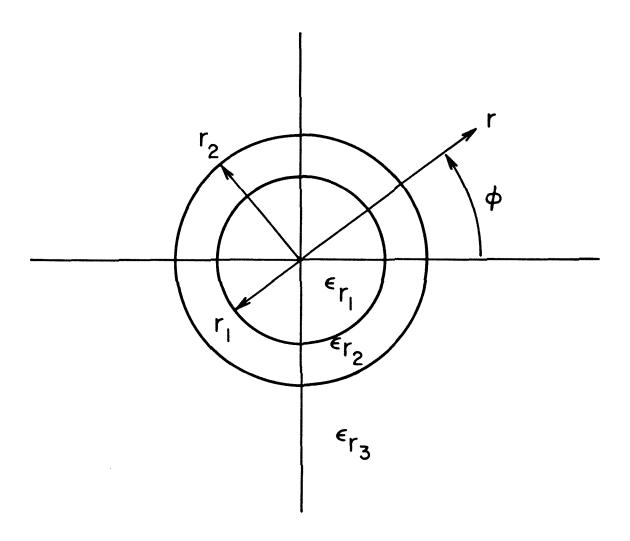
Figure I-1: Cross section of 3-region cylindrical dielectric waveguide
