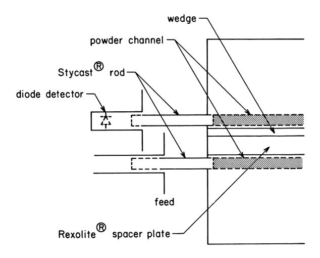
Figure IV-16: Top view schematic of the near end of the channel guide coupler during testing of the directivity
