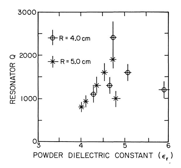
Figure III-4: Measured Q values of ring resonators versus the dielectric constant of the powder (Trans-Tech D-30 nickel aluminum titanate)
