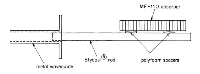
Figure IV-8: Setup for testing coupling between metal guide and dielectric rod
