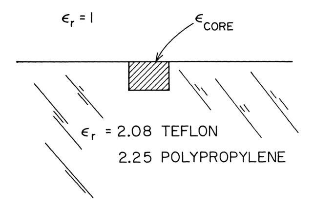
Figure II-1: Cross section of dielectric channel waveguide
