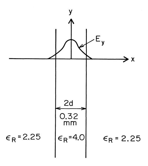
Figure AIV-1: Transverse cross section of the dielectric slab waveguide for which radiation losses were calculated. The electric field distribution is shown for the  $\mathrm{TE}_0$  mode.
