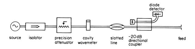
Figure IV-7: Setup of the X-band test equipment
