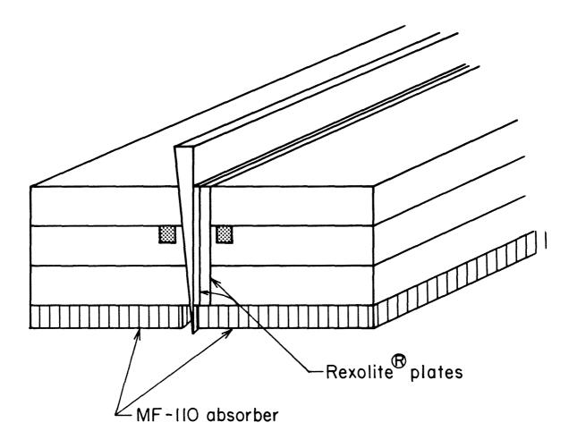
Figure IV-5: Diagram of coupled channel guides showing Rexolite  $^{\rm R}$  plates used to increase the range of separation distance possible with the experiment. Supporting structures (metal jacks) not shown.
