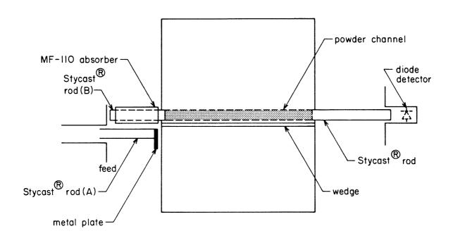
Figure IV-14: Top view schematic of setup for determining the power coupled onto the near end of the secondary channel guide
