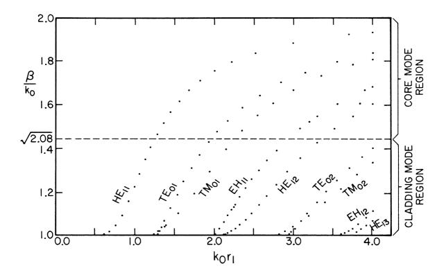
Figure I-3: Dispersion curves of 3-region cylindrical dielectric waveguide.  $\epsilon_{\rm r1}$  = 4,  $\epsilon_{\rm r2}$  = 2.08, and  $\epsilon_{\rm r3}$  = 1.  $r_2$  = 1.25  $r_1$ .
