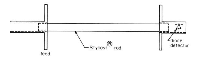
Figure IV-9: Setup for measuring the transmission loss of a dielectric rod
