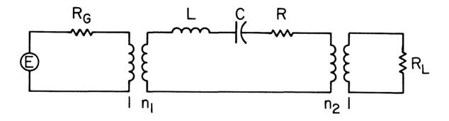
Figure AIII-1: Circuit model for a resonator used as a transmission filter
