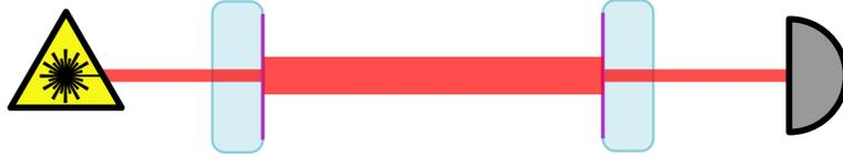
Figure 2.2: Diagram of a Fabry–Pérot interferometer. The photodiode may also be placed in so as to monitor the reflected light, rather than the transmitted light.
