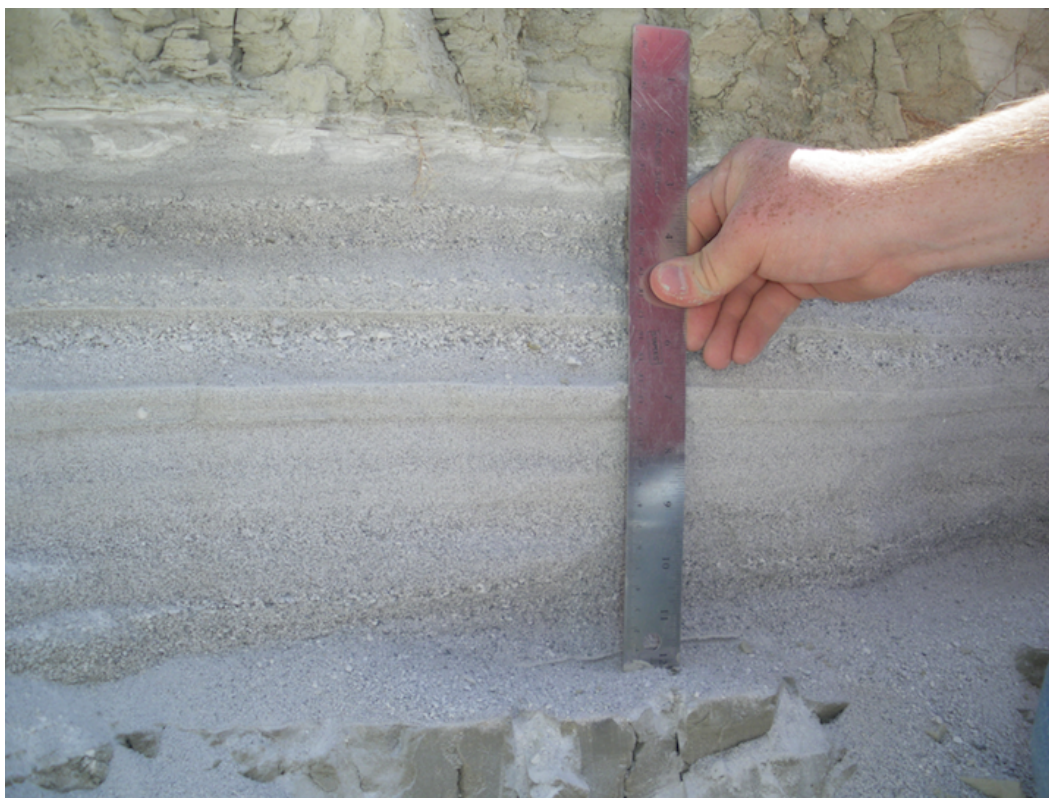
Figure 4.1: Ash 15 at the South Shore outcrop ( 37^{\circ}59'11''\text{N} , 118^{\circ}54'44''\text{W} ) after the outer weather layer was removed, shortly before sampling. The sampling location is the second layer from the top of the ash, which is the uppermost coarse layer.
