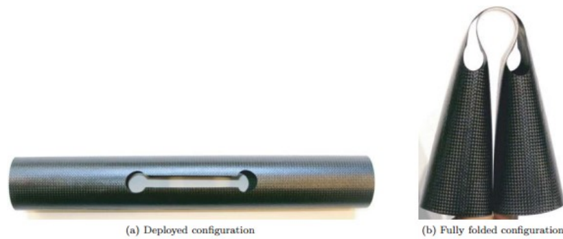
Figure 7.1: Image of an unfolded and folded material hinge in a carbon fiber composite tube. The hinge is created by simply removing a section of material from the tube. Source: [70].
