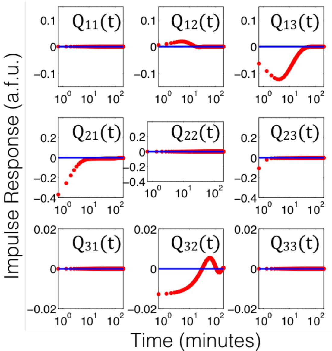
Figure 3.7: Impulse response of the estimated convolution kernel  $Q(t)$  matrix.  $Q(s)$  is estimated directly from experimental data, transformed into the frequency domain, and simulated in time for  $t = 0$  to  $t = 300$  minutes.
