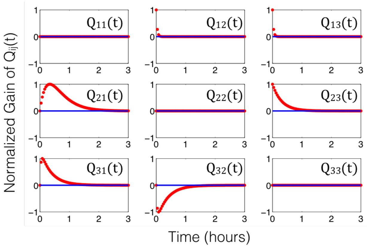
Figure 3.4: **Dynamical structure functions describe how network structure evolves over time (and as a function of frequency):** The time-lapse response of the dynamical structure convolution kernel  $Q^a(t) = \mathcal{L}^{-1}(Q^c(s))$  for the incoherent feedforward loop in system (3.6). By examining the functional response of each entry in  $Q(t)$  (or  $Q(s)$ ), we see that the network structure of the incoherent feedforward loop in Example 3.2.1 is a time-evolving, or *dynamic*, entity.
