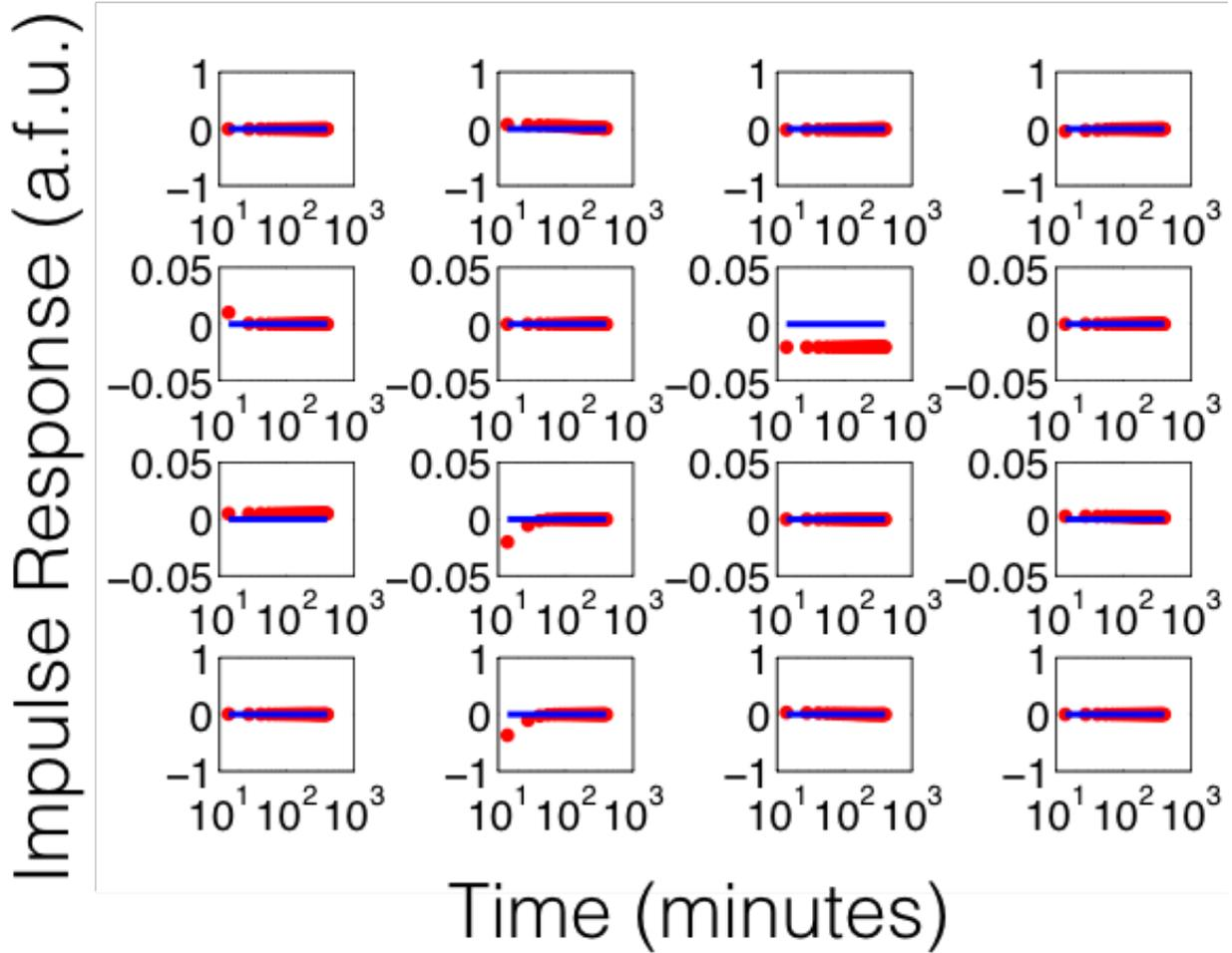
Figure 3.11: Impulse response of the estimated convolution kernel  $Q(t)$  matrix when the event detector biocircuit is induced with 1 nM HSL.  $Q(s)$  is estimated directly from experimental data, transformed into the frequency domain, and simulated in time, plotted in log-scale to make fast transients dynamics more visible.
