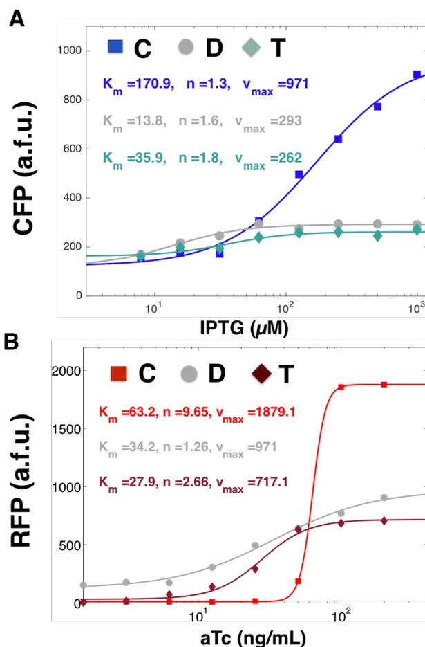
Figure 2.4: **Ultrasensitivity, basal expression, and amplitude of gene induction responses are significantly affected by compositional context:** (A) Induction curves for convergent-, divergent-, and tandem- oriented CFP fitted to a Hill function at aTc = 200 ng/mL and varying concentrations of IPTG. (B) Induction curves for convergent-, divergent-, and tandem-oriented RFP fitted a Hill function at IPTG = 1000 nM and varying concentrations of aTc.
