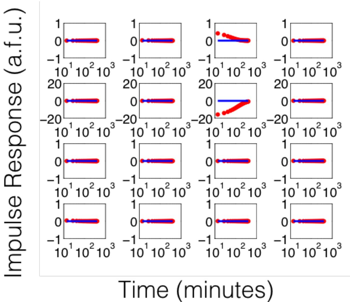
Figure 3.13: Impulse response of the estimated convolution kernel  $Q(t)$  matrix when the event detector biocircuit is induced with  $1 \mu\text{M}$  HSL.  $Q(s)$  is estimated directly from experimental data, transformed into the frequency domain, and simulated in time, plotted in log-scale to make fast transient dynamics more visible.
