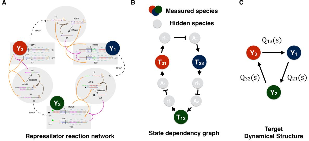
Figure 3.5: **Network representations of a synthetic genelet repressilator:** (A) A reaction network using push-arrow reaction notation of the synthetic genelet repressilator. (B) A diagram representing the reaction dynamics in panel (A) as state dependencies from a nonlinear ODE model in [49]. (C) The dynamical structure of the repressilator (without inputs), with nodes representing measured chemical species and edge weights corresponding to entries in  $Q(s)$ .
