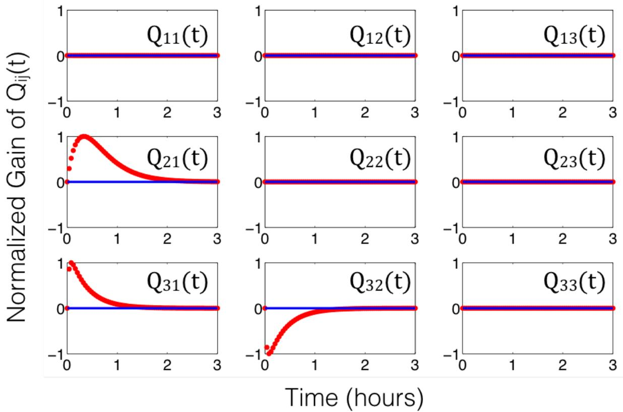
Figure 3.2: **Dynamical structure functions describe how network structure evolves over time (and as a function of frequency):** The time-lapse response of the dynamical structure convolution kernel  $Q^a(t) = \mathcal{L}^{-1}(Q^a(s))$  for the incoherent feedforward loop in system (3.6). By examining the functional response of each entry in  $Q(t)$  (or  $Q(s)$ ), we see that the network structure of the incoherent feedforward loop in Example 3.2.1 is a time-evolving, or *dynamic*, entity.
