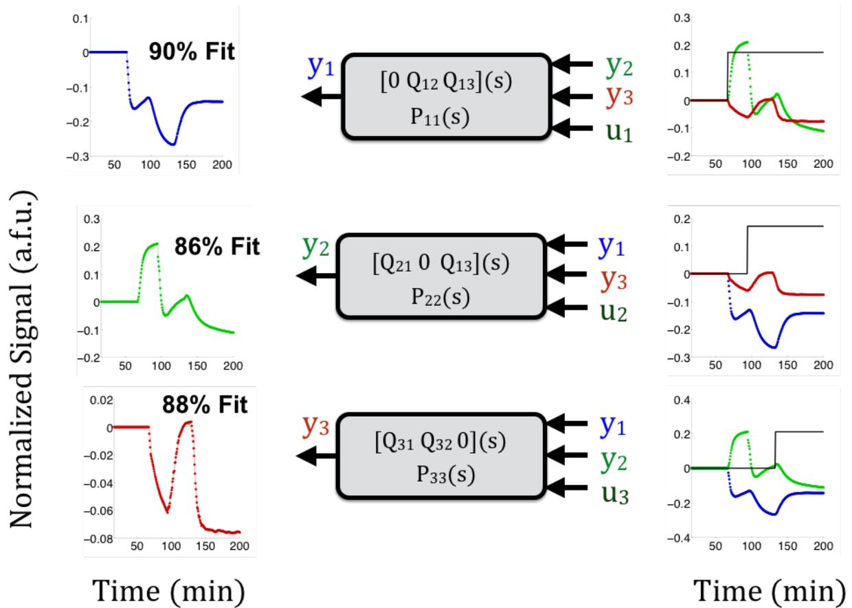
Figure 3.6: Time-series experimental data from *in vitro* network perturbation experiments of a T7 RNAP genelet repressilator. Three outputs are measured simultaneously,  $y_1$ ,  $y_2$ , and  $y_3$ , corresponding to DNA switches  $T_{31}$ ,  $T_{12}$  and  $T_{23}$ . DNA homologues of the RNA inhibitors  $rI_j$   $j = 1, 2, 3$  are injected at small concentrations to provide a step input perturbation to the corresponding component  $Y_j$  in the genelet circuit.
