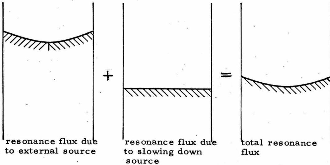
Fig. 8. Schematic illustration of the resonance flux for a mixture of nuclei.
