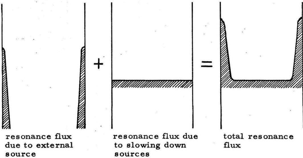
Fig. 6. Schematic illustration of the resonance flux for  $\Gamma_\gamma/\Gamma$  large.
