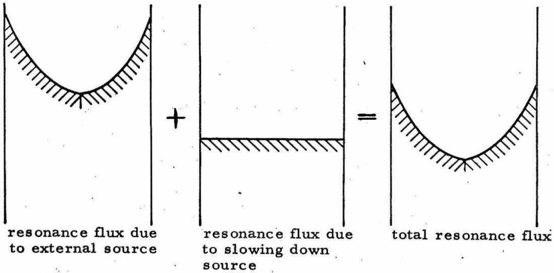
Fig. 7. Schematic illustration of the resonance flux for  $\Gamma_y/\Gamma$  small.
