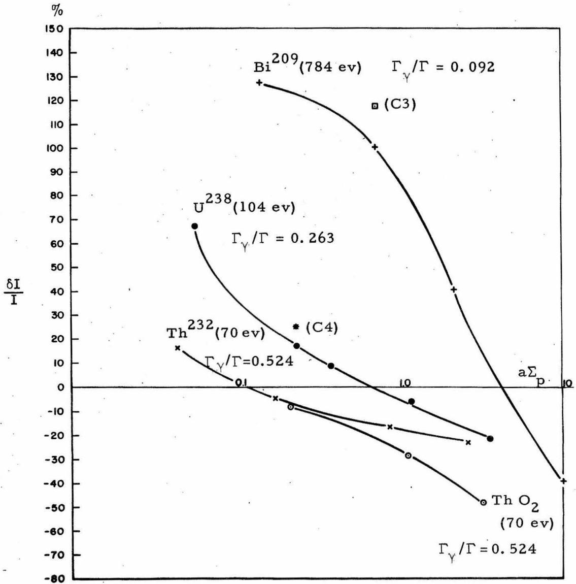
Fig. 22. Fractional error introduced in the resonance integral by the infinite mass approximation.
