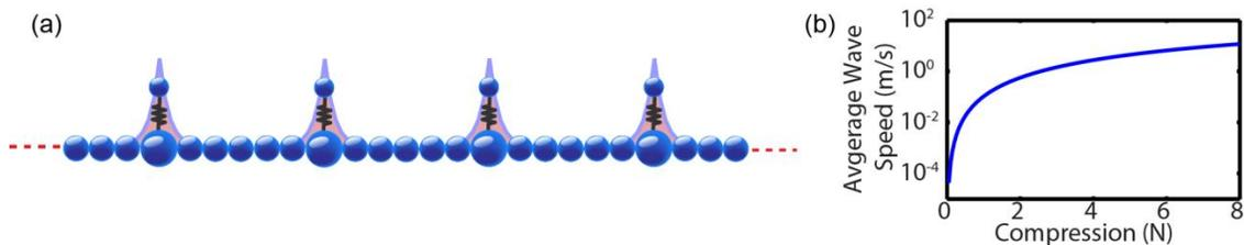
Figure 5.5: Ultraslow velocity wave propagation. (a) A design proposal for achieving tunable ultraslow acoustic or phononic propagation. (b) The wave velocity of the
