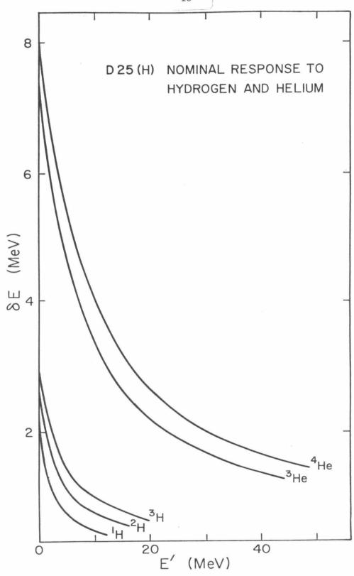
Since the calculated mass,  $M(\delta E, E', t)$  is a function of the energy loss, residual energy and assumed thickness of the first detector, the mass resolution is determined by the uncertainty in  $\delta E$ , E' and t. The sources of error in each of the quantities are now considered.
