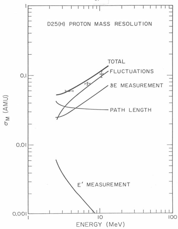
D2, the value of  $\delta E$  becomes much higher than normal. As Figure II-2 suggests, such a proton might be interpreted as a higher mass particle.
