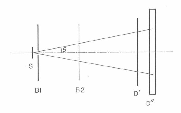
varying the distance between B1 and B2, the angle  $\theta$  can be adjusted. By removing the solid centre of baffle, B2, all angles up to  $\theta$  can be included in the beam. In all cases the beam illuminates only the fully active areas of D' and D". D' and D" are simultaneously pulse height analysed by the 'PACE system' electronics (Marshall, 1974b), with individual pulse height pairs recorded on tape. The effective channel widths of 40 key are similar to those used for D2 and D5.
