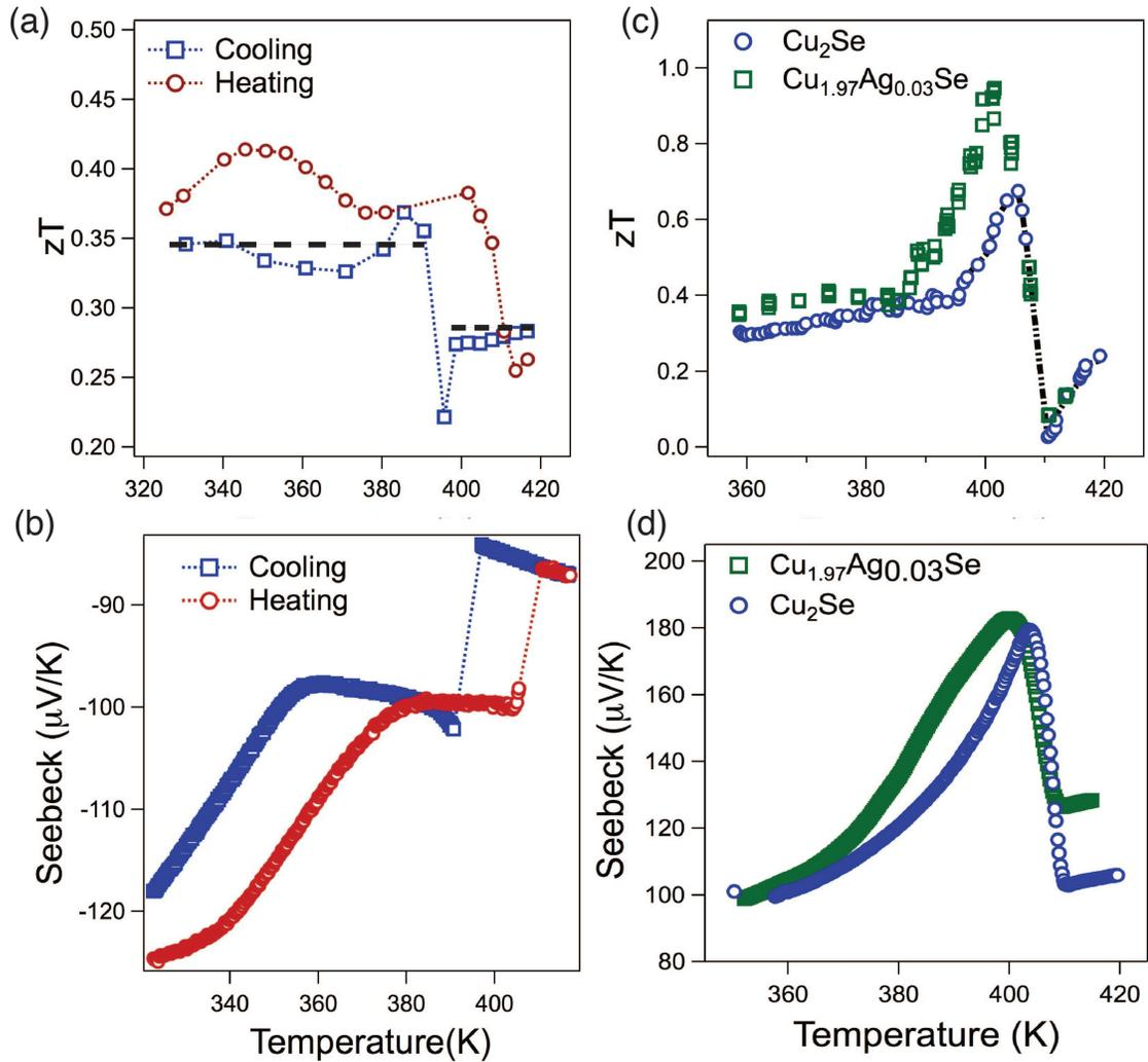
Figure 8.1: Key results of this thesis. Concurrent with its first order transition there is a step change in  $\text{Ag}_2\text{Se}$   $zT$  (a) and Seebeck (c). The second order transition of  $\text{Cu}_2\text{Se}$  results in a sharply peaked  $zT$  (a) and Seebeck (d). The  $zT$  and Seebeck of the mixed phase transition of  $\text{Cu}_{1.97}\text{Ag}_{0.03}\text{Se}$  resembles that of its  $\text{Cu}_2\text{Se}$  main phase. Dotted lines are guides for the eye.
