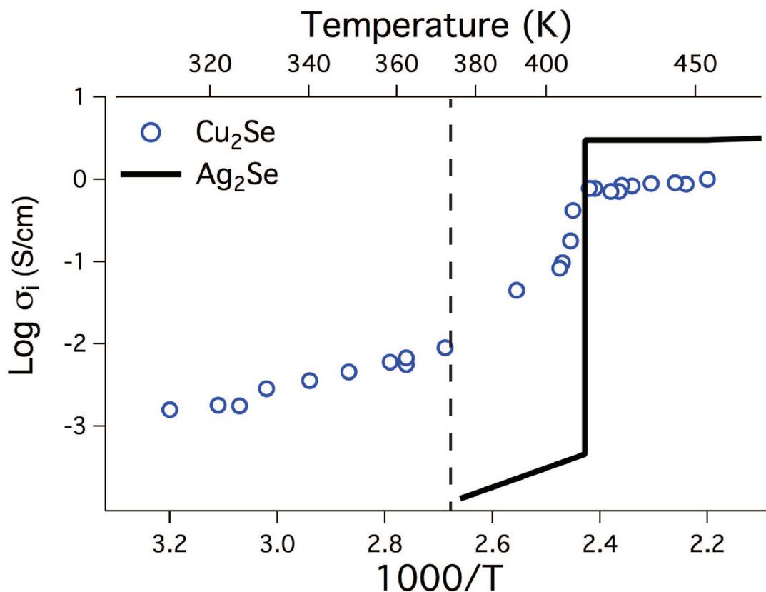
Figure 8.2: Ion conductivity of  $\text{Cu}_2\text{Se}$  [84] and  $\text{Ag}_2\text{Se}$  [136] through their phase transitions.  $\text{Ag}_2\text{Se}$  shows a step increase in ion conductivity at its phase transition, while  $\text{Cu}_2\text{Se}$  shows a super-exponential increase in ion conductivity to the phase transition temperature. The dotted line corresponds to 374 K, at which temperature the super-exponential increase begins.
