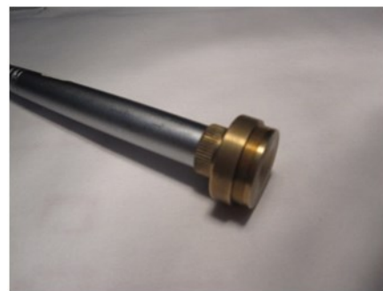
b) Connected with B&K Type 2669 Preamplifier.
