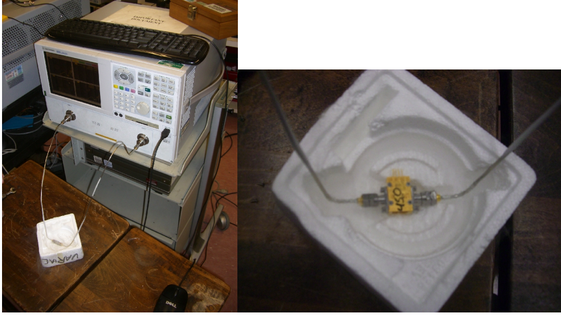
Figure 7.23: Measurement setup for cryogenic capacitor tests
