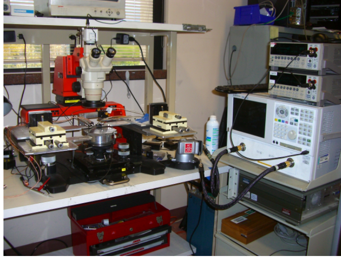
Figure 7.1: Photograph of the test setup for wafer-probed S -parameter measurements at 300 K. The bias is provided using three Keithley KE2400 DC supplies, one of which is not shown in the photo.
