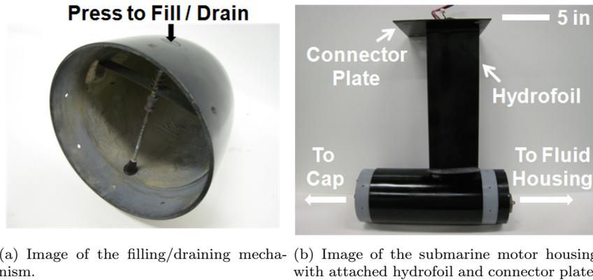
(a) Image of the filling/drainage mechanism. (b) Image of the submarine motor housing with attached hydrofoil and connector plate.
