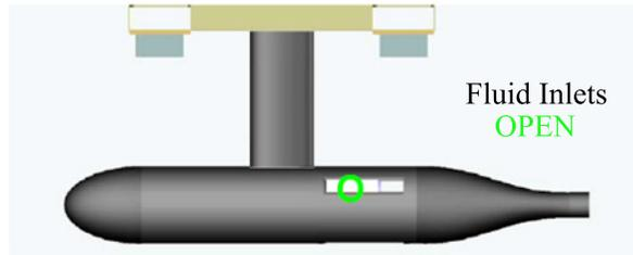
Figure 2.9. Principle of operation for steady jet configuration.
