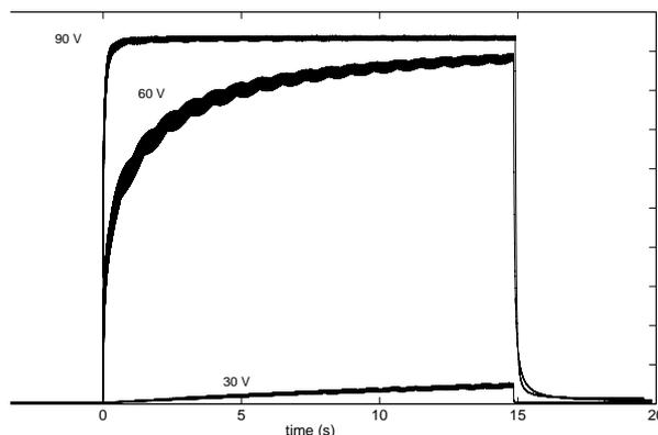
Figure A.1: Response of a 5 wt % gel in a  $15\mu$  gap to an external voltage of 30 V, 60 V, and 90 V. The voltage is applied at 0 s and removed at approximately 15 s.
