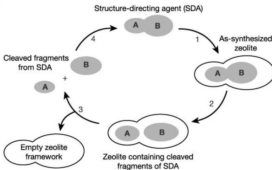
**Figure 5.4** Recyclable structure-directing agent route – (1) zeolite synthesis; (2) cleavage of the organic molecules inside the zeolite pores; (3) removal of the cleaved fragments; (4) recombination of the fragments into the original SDA molecule<sup>2</sup>
