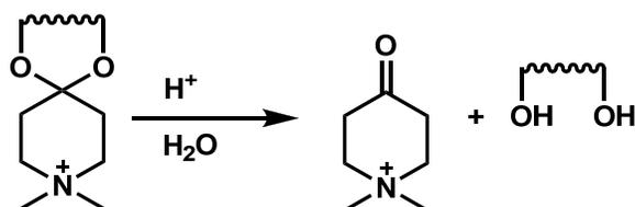
**Figure 5.3** Cleavage reaction of ketal-containing structure-directing agent into smaller fragments<sup>21</sup>
