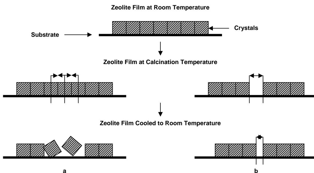
**Figure 5.1** Schematic representation of the results of thermal stresses on zeolite films during calcination: (a) cracking at film / substrate interface if film is not well-adhered to substrate, (b) cracking within film if film is well-adhered to substrate
