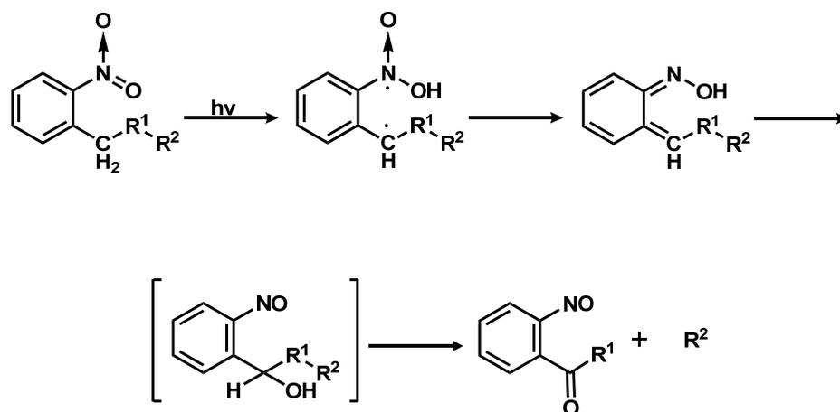
**Figure 5.7** Schematic of the 2-nitrobenzyl group cleavage mechanism via hydrogen abstraction
