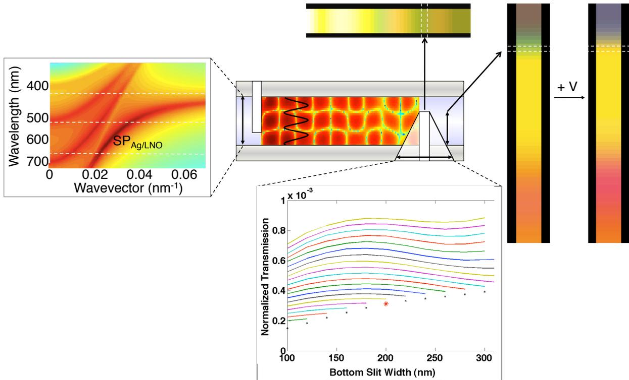
Figure 9.1. Methods for modifying the output of the MIM color filters included: varying the thickness (left); varying the depth of the output slit with and without an applied electric field (right); varying the separation between the input and output slits (top); varying the shape of the input and output slits (bottom). Representative one and two-dimension mode profiles are shown within the waveguide cavity.
