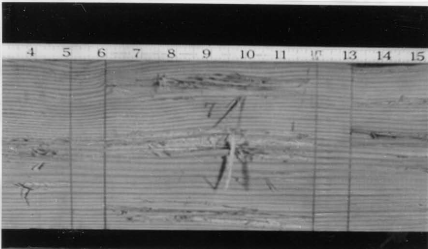
SAMPLE AFTER 20 SURGE TESTS (4000 AMPERES CREST)
