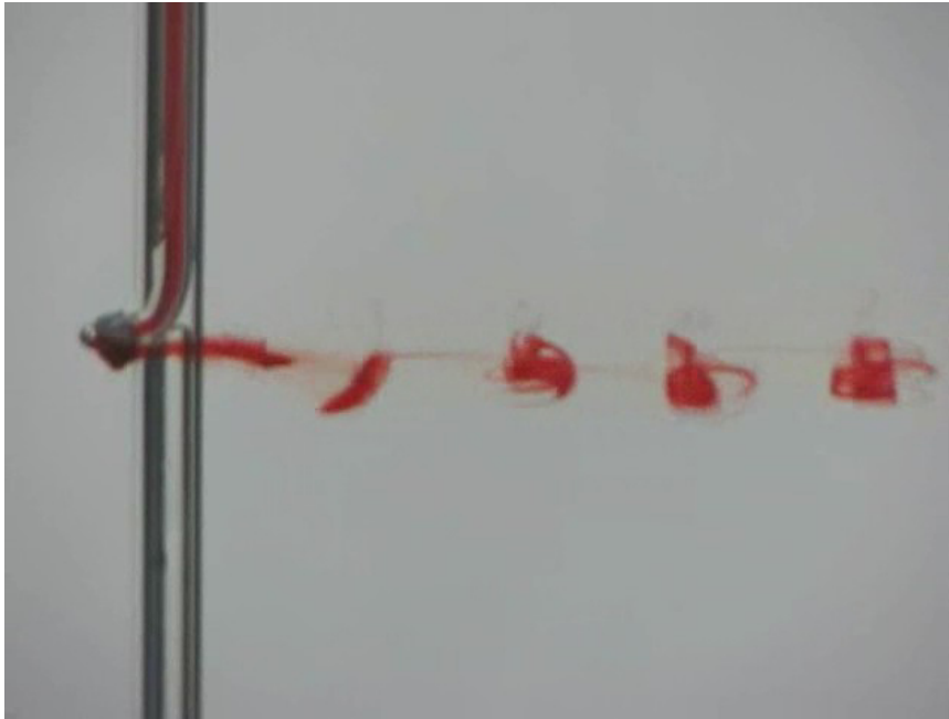
Figure 5.12: Flow visualization showing the nearly two-dimensional flow around an oscillating cylinder at its maximum amplitude, A_{\text{Max}}^* \approx 0.35 , for \text{Re} \approx 200 .
