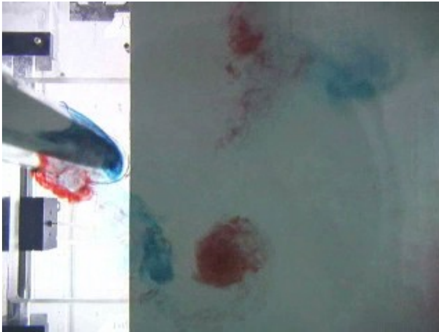
Figure 4.23: Flow visualization of the wake during an individual cycle of the middle of the upper branch (case 3) showing a structure resembling a classic 2P wake.
