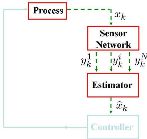
Figure 1.2: State Estimation over a Wireless Sensor Network
