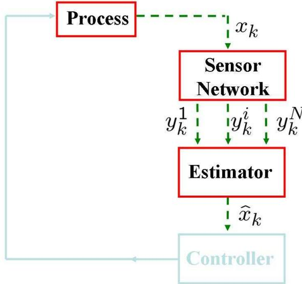
Figure 3.1: State Estimation Using a Wireless Sensor Network
