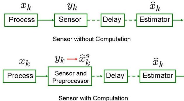
Figure 1.3: State Estimation over a Packet Delaying Network
